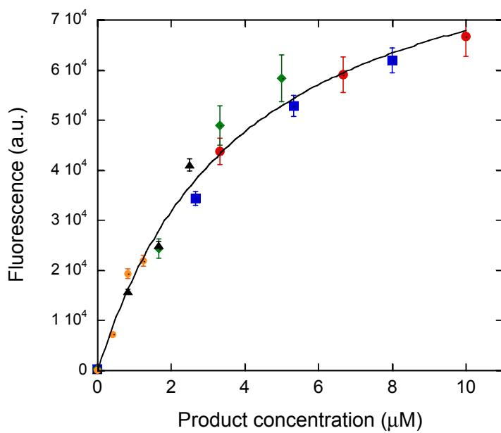
Fig. S1      Fluorescence detection in the PμD device. Each set of data corresponds to specific flow rates: ● = 10, 10, 10, 10 (for oil, buffer, fluorescein 15  $\mu\text{M}$  and *E. coli* alkaline phosphatase respectively, expressed in  $\mu\text{l}\cdot\text{h}^{-1}$ ), ■ = 10, 8, 8, 14 and ◆ = 10, 5, 5, 20; ▲ = 10, 10, 10, 10 (for oil, buffer, fluorescein 3.75  $\mu\text{M}$  and *E. coli* alkaline phosphatase respectively, expressed in  $\mu\text{l}\cdot\text{h}^{-1}$ ).
