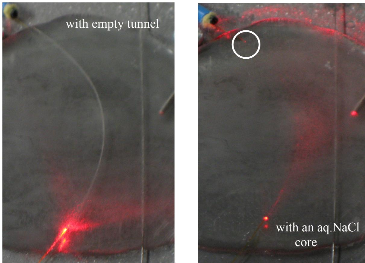
Fig.S-1 Light guiding with curved water-ice LCW.
