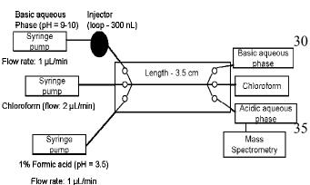
A visual representation of three-phase microchip extraction efficiency 30 at a flow rate of 0.5:1:0.5  $\mu$ L/min flow rate, 12.5 sec residence time
