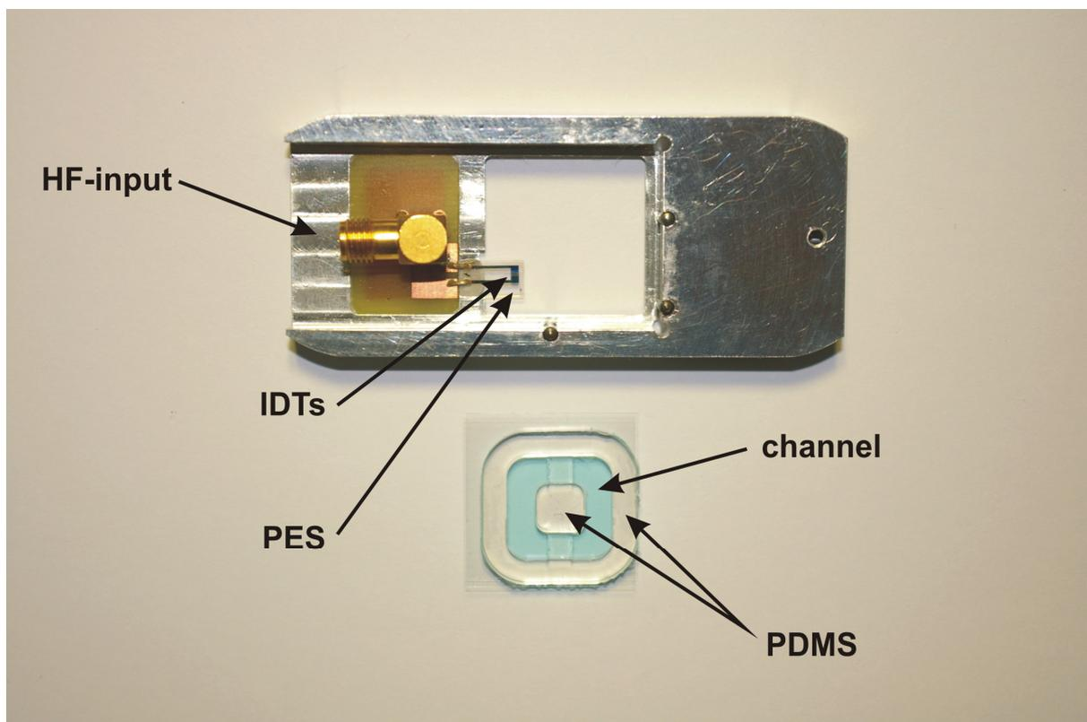
**Figure S4.** Interdigital transducers (IDTs). Bar represents 100  $\mu\text{m}$ .
