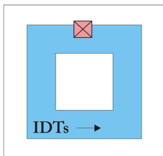
**Figure S3.** Acoustically-driven biochip and 3D-microchannel. Surface acoustic wave (SAW) pump consisting of the high frequency connector (HF-input) and piezoelectric substrate (PES) with interdigital transducers (IDTs).
