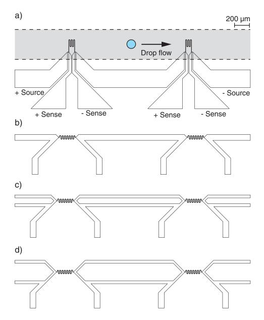
**Figure S-2.** Drawings, to scale, of the sensors from different PRTD array designs. The scale bar in drawing a) applies to all drawings. Drawing a) also shows the outline of a 400-μm wide channel aligned with the array.
