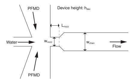
**Figure S-1.** The critical geometrical design parameters of the microfluidic devices used for the freezing of water drops.
