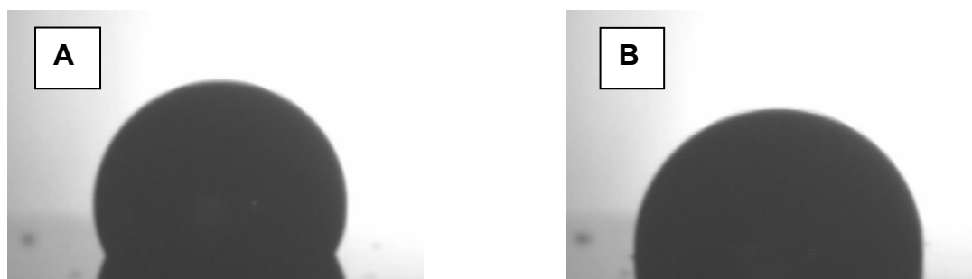
Figure S1: Experimental results of the contact angle measurements as described in the Experimental section. A: 0V, 116° B: 450V, 91.5°. Contact angles were analyzed with the contact angle measurement tool of the free image analysis software package ImageJ, with an estimated uncertainty of 0.5° due to placement of the baseline for B.
