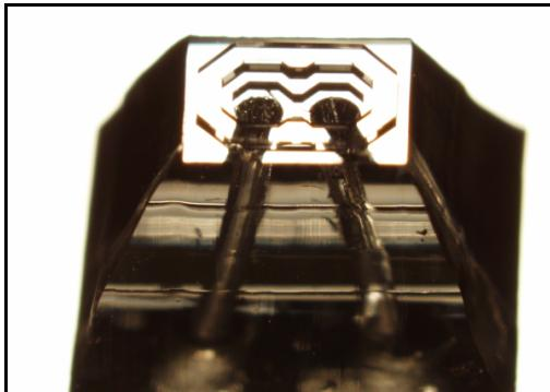
The polystyrene (PS) support layers were 1 centimeter squares cut from standard disposable petri dishes using a heated razor blade. Holes were drilled a few millimeters apart with a drill press to accept 28-gauge PTFE tubing for the fluid
