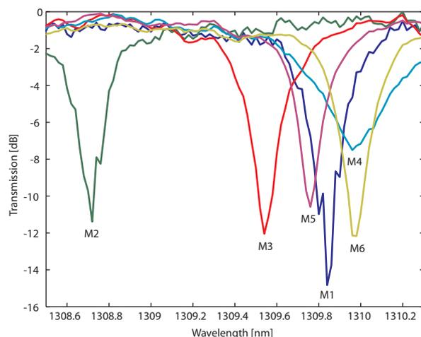
**Figure S3:** A superposition of the concurrently collected transmission spectra of resonators M1 to M6 operating in phosphate buffered saline (PBS) at a laser input power of 9 mW. The ring resonators display a throughput attenuation of -7 to -15 dB, a quality factor of a few thousand, and a free spectral range of 2.2 nm.
