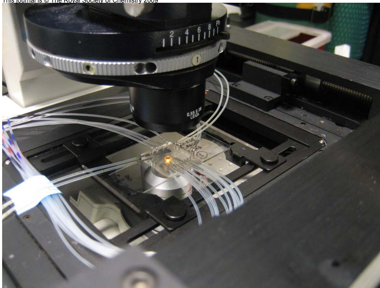
ESI Figure 2. Array device mounted to microscope stage. Line of 10 L-shaped steel pins are inserted into ports for on-chip valve control channels. Other pins are inserted into flow ports. Dimensions of PDMS device are 25 x 25 x 4 mm. Underlying substrate is a 25 x 75 x 1 mm glass slide. For high magnification observation (40X+), a glass cover slip can be used as the substrate.
