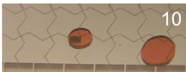
**Figure 1S:** Frames from a movie depicting passive dispensing onto an adhesion pad. In frames 1-5, a yellow droplet is dispensed onto a dry pad, and in frames 6-10, the yellow droplet is replaced with a red droplet. The source and dispensed droplet volumes were 1  $\mu\text{L}$  and  $\sim 150$  nL.
