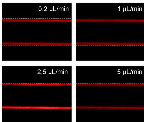
Superimposed images confirming the margination of 6 μm beads (fluorescently labeled red) to the channel sidewalls at the microchannel outlet. Tests were conducted with a 40% hematocrit sample spiked with fluorescently labeled beads at flow rates ranging from 0.2 μL/min to 5 μL/min. (white dotted lines indicate the approximate channel wall boundaries).
