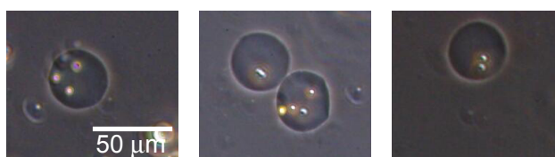
Fig. S2. Encapsulation of solid particles as a model of cells. Fluorescent solid particles were encapsulated into the calcium alginate microbeads. Images were captured using a phase-contrast and fluorescent microscope.
