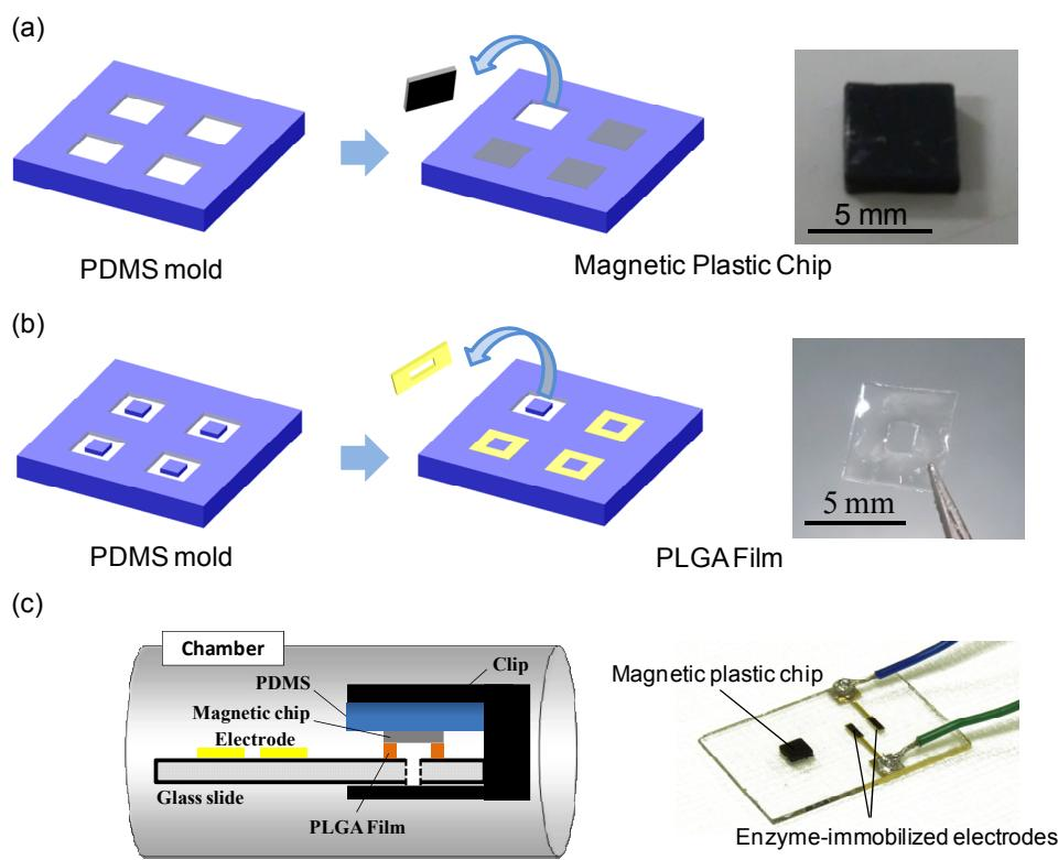
Supplementary Figure 1. Fabrication process and photographs of (a) magnetic plastic chip, (b) PLGA film and (c) the magnetic chip bonding to an enzyme-immobilized glass slide via a PLGA film.
