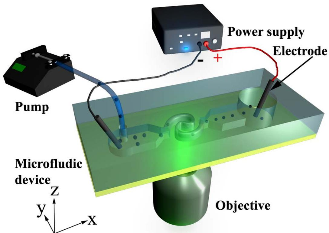
**Figure S1.** A schematic illustration of the setup of flow-through electroporation. The drawing is not to scale and the layout of the narrow section is simplified for drawing convenience.
