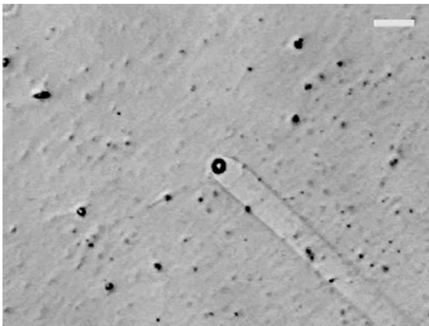
**Movie S1.** Real-time movie of data shown in Figure 2a. The orientation of a 6% (w/v) BSA stream emerging from the central pore is switched by successive activation of eight solenoid pinch valves for 1 s each. The entire cycle was repeated twice. Data was acquired at 2 Hz. Scale bar, 20  $\mu\text{m}$ .
