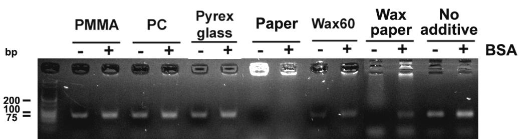
**Fig. S1** PCR biocompatibility with materials used in the study. The reaction outcome can be seen in PCR with and without BSA.
