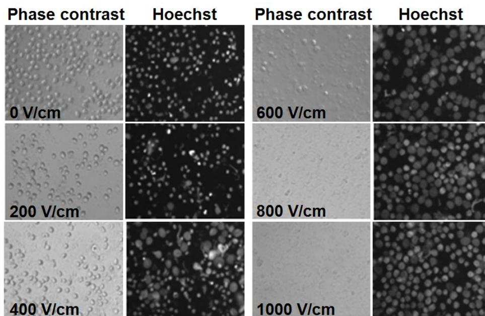
**Figure S1.** Electroporation of Hoechst 33342 (Invitrogen) stained DT40 cells at different field strengths. The field duration is 100 ms. *The images indicate that the nuclei stay in the cells with field intensity up to 1000 V/cm.*
