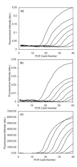
**Fig. S2** On-cartridge real-time PCR. The real-time fluorescence curves of serial diluted (1–10<sup>6</sup> folds) GAPDH cDNA, amplified and measured with (a) the custom-built thermal cycler, (b) the MJ Research Opticon system, and (c) the Bio-Rad CFX96 system. The custom-built thermal cycler utilized LEDs as light source and a PMT for detection, the MJ Research Opticon system employed LEDs plus PMTs, and the Bio-Rad CFX96 system used LEDs and photodiodes.
