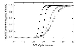
**Fig. S3** On-cartridge real-time PCR. The real-time fluorescence curves of serial diluted (( $\bullet$ ) 0-fold, ( $\bullet$ ) 10-fold, ( $\circ$ ) 10<sup>2</sup>-fold and ( $\Box$ ) 10<sup>3</sup>-fold) influenza A, amplified and measured with the custom-built thermal cycler and detection system.
