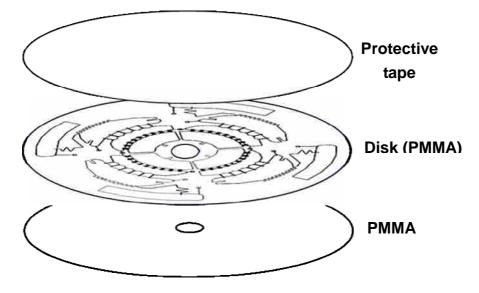
**Fig. S1.** Sketch of the three-layer disk assembly. A  $CO_2$  laser engraver was used to cut the 1mm thick PMMA disk (middle layer) with microfluidic features. Then, the disk was bonded with a plain PMMA plate as substrate and a top layer of protective tape for enclosure.
