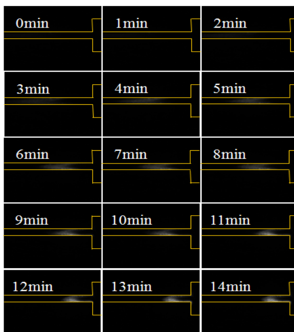
Fig. 2s Temporal sequential microscopic fluorescence images for sample solute concentration experiment using microfluidic Joule heating induced temperature gradient focusing technique. In the experiment, a solution containing 0.05\mu\text{M} Fluorescein-Na solutes dissolved in a 180 mM Tris-borate buffer is loaded into a 10mm-long PDMS microchannel with two square-shaped reservoirs of 16\text{ mm} \times 16\text{ mm} . Once a combined 400\sin(2\pi ft) V AC and 450 V DC field is imposed to the two reservoirs with the left-hand side grounded, the sample solutes are gradually focused at a stagnant point in the narrow channel region.
