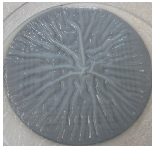
Fig. S2 SIFEL cured as a thick layer. The top surface is wrinkled with a thickness varying up to an order of magnitude.
