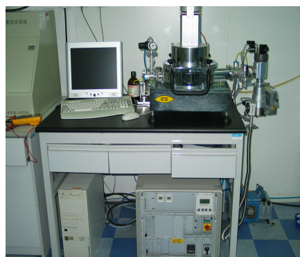
Figure E2 A photograph of EVG-501 bonding equipment. This is a wafer-level bonding apparatus manufactured by EVG Company. Parameters including bonding temperature, pressure, voltage and contact force for anodic bonding could be tuned at this apparatus.
