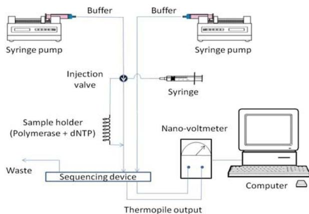
**Fig.S1.** Two Harvard Apparatus syringe pumps inject 1xPolymerase buffer solution into the inlet ports of the microfluidic device. The sample is injected to the buffer stream supplied to Inlet 2 using a 6-Port injection valve. The thermopile voltage is measured using a nanovolt meter and the signal is recorded using LabView SignalExpress software.
