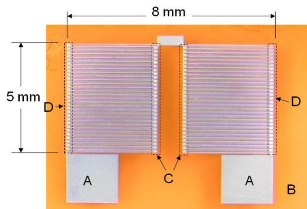
**Fig.S2.** Antimony/Bismuth thermopile with 60 thermocouple junctions (A = contact pads, B = polyimide support, C = measuring junctions, D = reference junctions).
