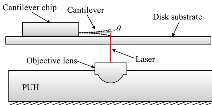
Figure S2. The angular tolerance of the DVD measurement platform.
