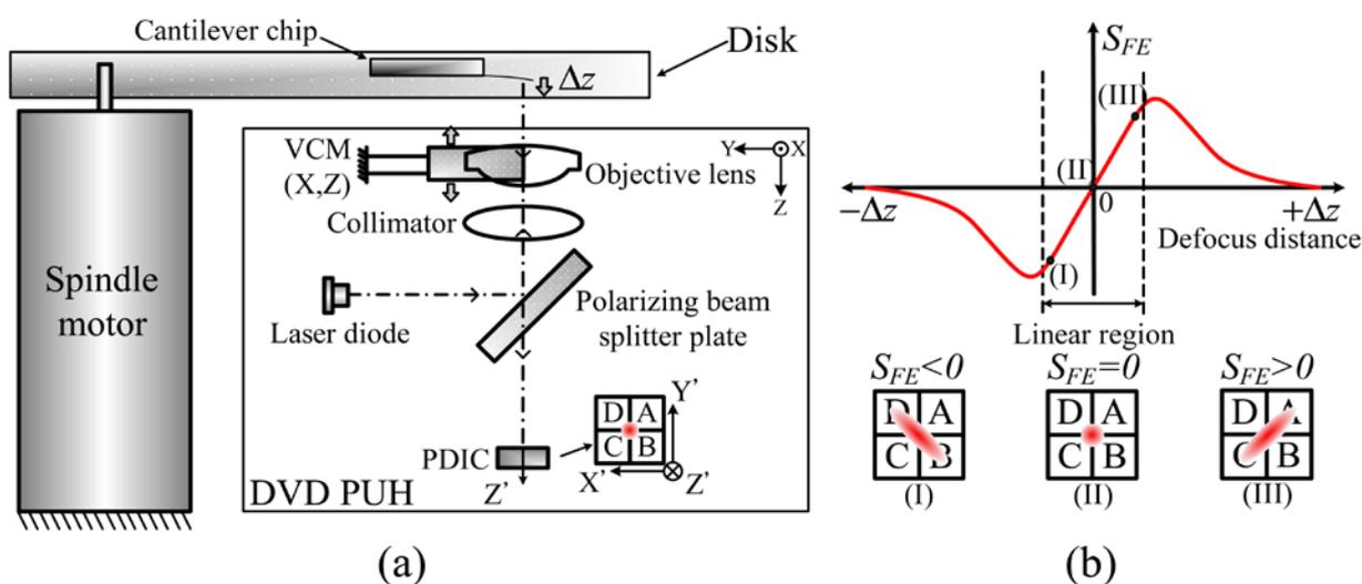
Figure S1. The detection scheme of the cantilever read out system. (a) Schematic diagram of the system. (b)  $S_{FE}$  vs. defocus distance
