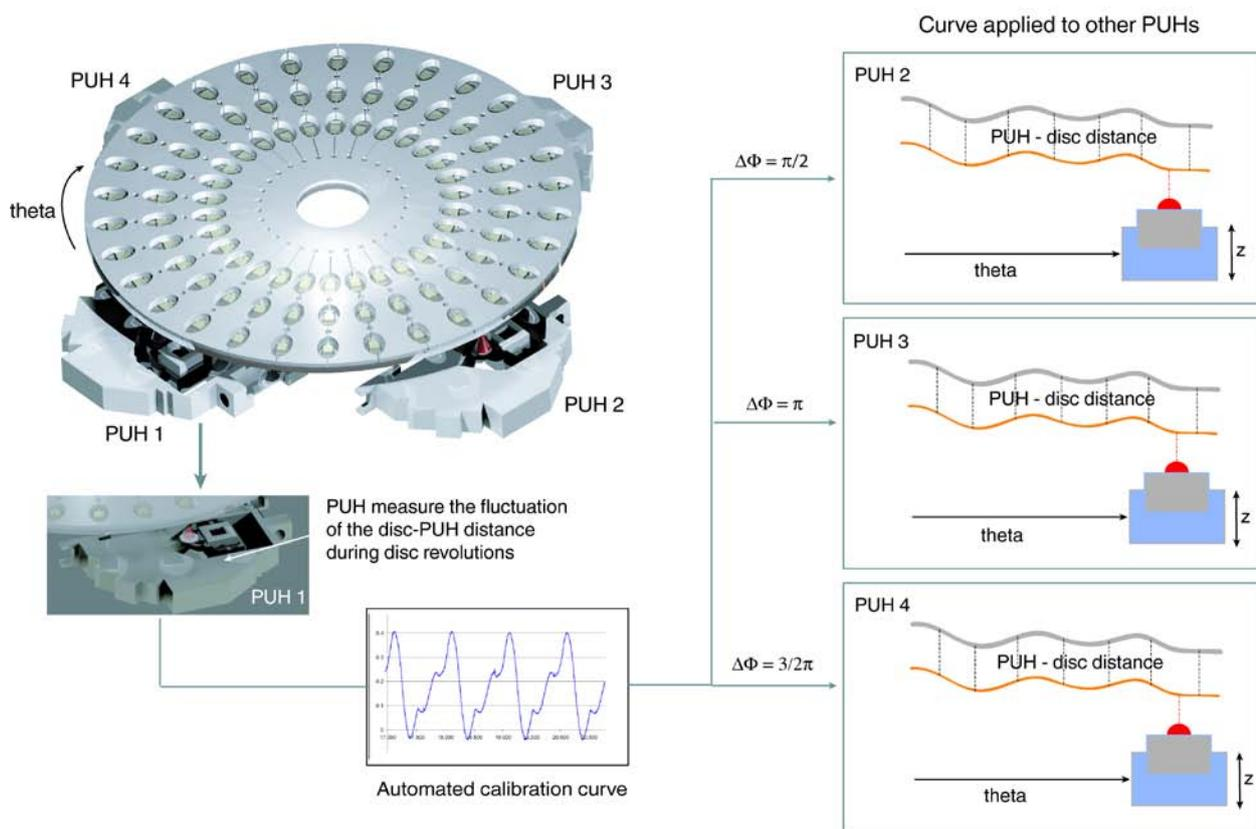
Figure S3. Scheme of the 4-PUH auto-calibration approach.
