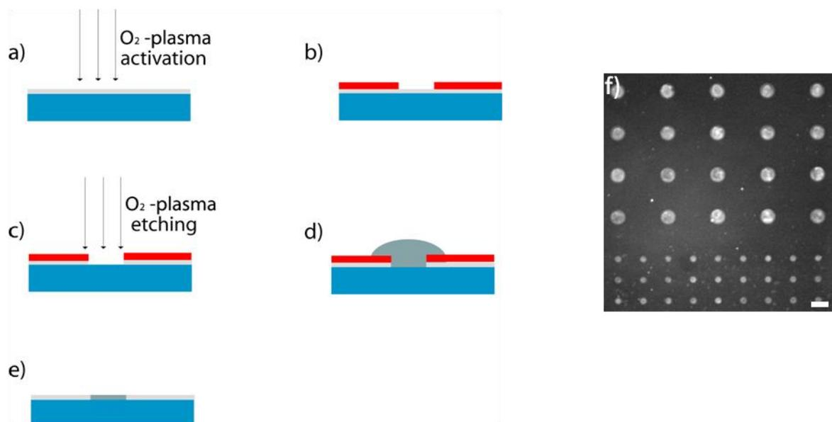
**Figure S1** Schematic drawing of the wet lift-off method for functionalizing of EWOD digital microfluidic chips: a) O<sub>2</sub>-plasma activation of the Teflon-AF<sup>®</sup> surface, b) photolithography, c) O<sub>2</sub>-plasma etching of exposed Teflon-AF<sup>®</sup>, d) seeding biomolecules, e) lift-off of sacrificial photoresist in ethanol, and f) fluorescent image of PLL-FITC micropatterns in a Teflon-AF<sup>®</sup> coated substrate as generated with the WLO method (scale bar = 50 μm).
