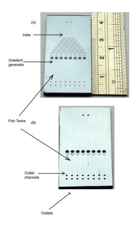
Supplementary 1: Fabricated chips: The top (B) and bottom (A) views of the chip are shown here with etched inlets, gradient generator, outlet channels and outlets
