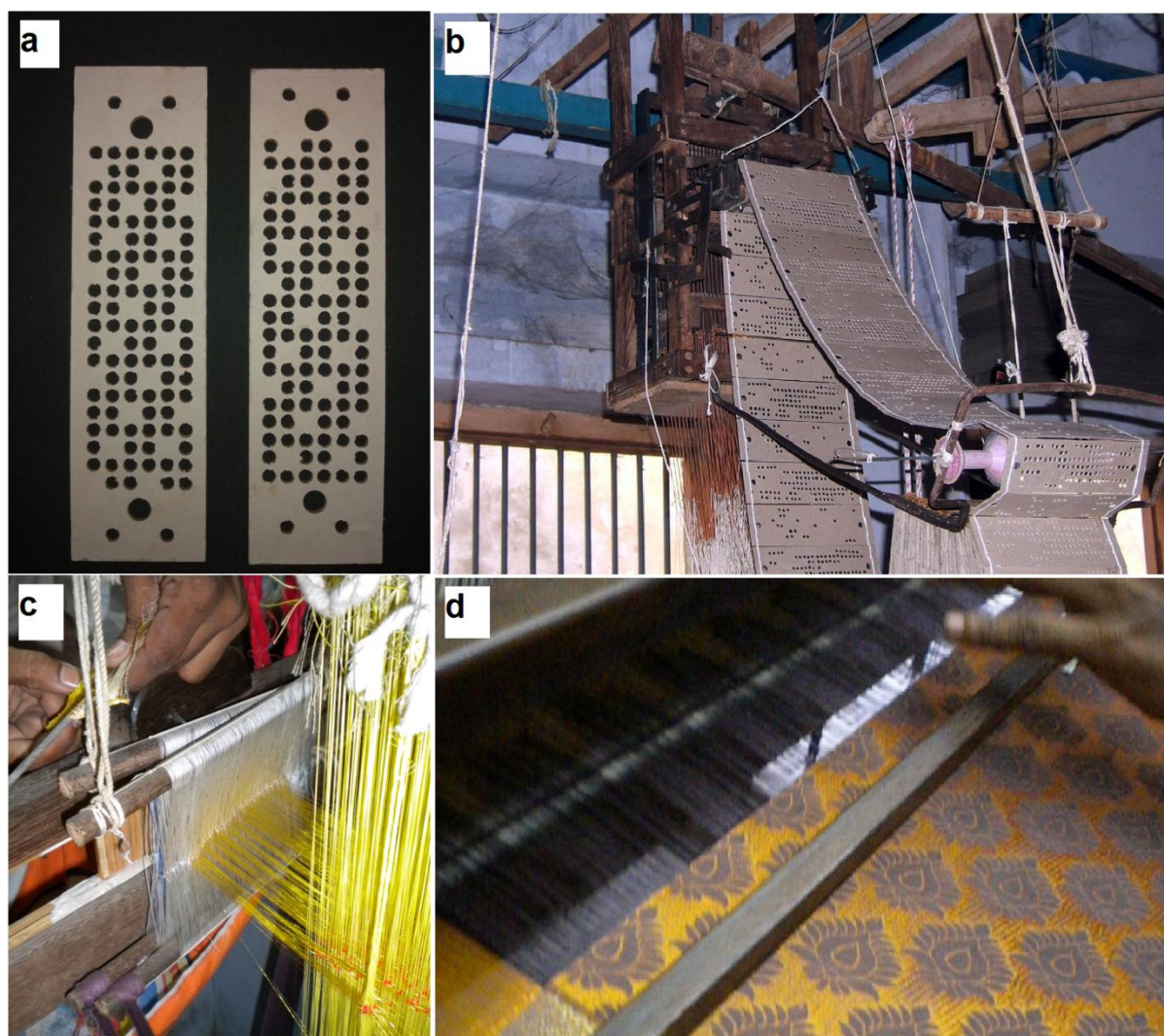
Fig. 1: Individual punched cards (a) are strung together into a series of several hundred punch cards and fitted into the Jacquard (b). The yellow hanging threads in (c) correspond to a set of hooks that can either be raised or stopped depending on the presence or absence of a punched hole in the card. The hook serves to raise or lower a harness that in turn raises or lowers a set of warp threads. Any number of warp threads may be simultaneously raised or lowered so that the pattern can be repeated across the fabric (d).
