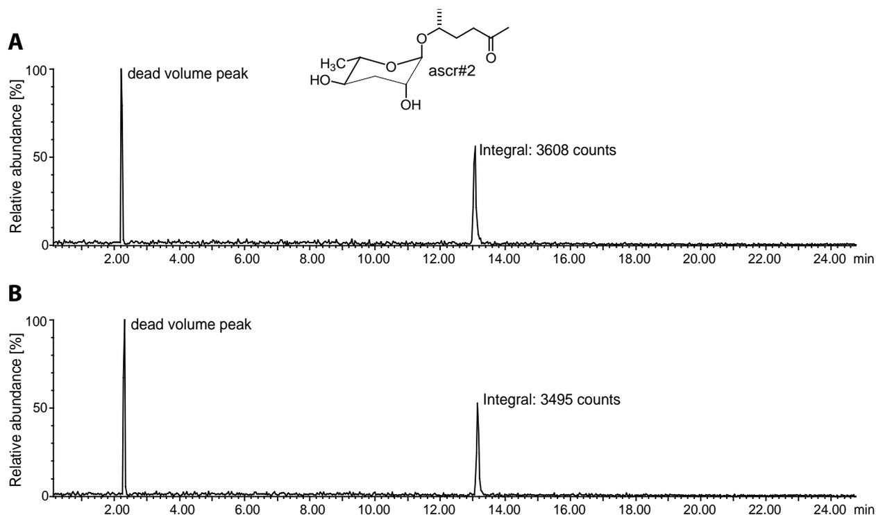
**Figure S3.** HPLC-MS ion chromatograms for the ion  $m/z = 269$ , corresponding to  $[M+Na]^+$  of ascaroside ascr#2. **A:** HPLC-MS ion chromatogram obtained with injection of 1  $\mu\text{L}$  of a 10  $\mu\text{M}$  solution of ascr#2 in water. **B:** HPLC-MS ion chromatogram obtained with injection of 1  $\mu\text{L}$  of the same solution after pass through microfluidic device. Integration of the peaks representing ascr#2 using MassLynx software (Waters) indicated less than 5% loss.
