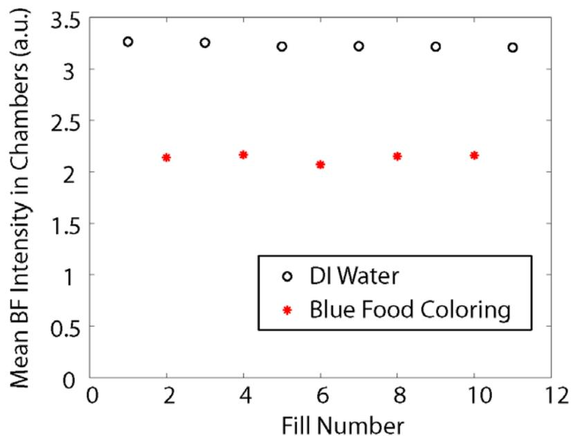
**Figure S1.** Repeated loading of DI water and blue food coloring into the device using a syringe pump operated at 0.3 ml/min. 100  $\mu$ L of solution was injected for each loading cycle. We observed that the chambers reach steady state concentration after 50  $\mu$ L injections.
