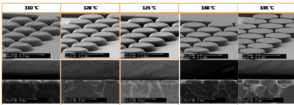
**Figure S4.** Cross-section SEM images of the micropillars fabricated in this study using microinjection molding. The pillar edge becomes sharper with increasing mold wall temperature, which means good replication quality.
