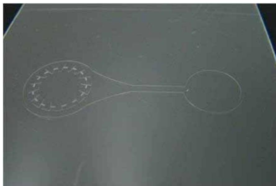
**Figure S2.** Image of the LOC prepared using microinjection molding. The micropatterns are constructed on the COC device.
