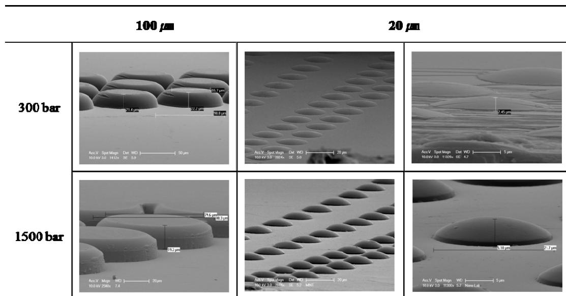
**Figure S3.** Effect of the packing pressure on the moldability for micropillars in the microinjection molding process. The mold filling quality of 20  $\mu\text{m}$  and 100  $\mu\text{m}$  micropillars were examined by comparing the SEM images of the pillars prepared under different packing pressures, i.e., 300 bar and 1500 bar.
