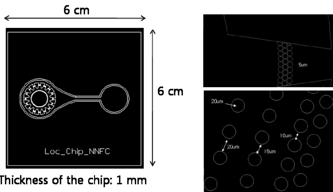
**Figure S1.** Schematic diagram of microstructured lab-on-a-chip (LOC). The left-hand image shows the entire dimension of the LOC device. The top-right image shows outer circle group micropillars, whereas the bottom-right images display the inner circle group micropillars.
