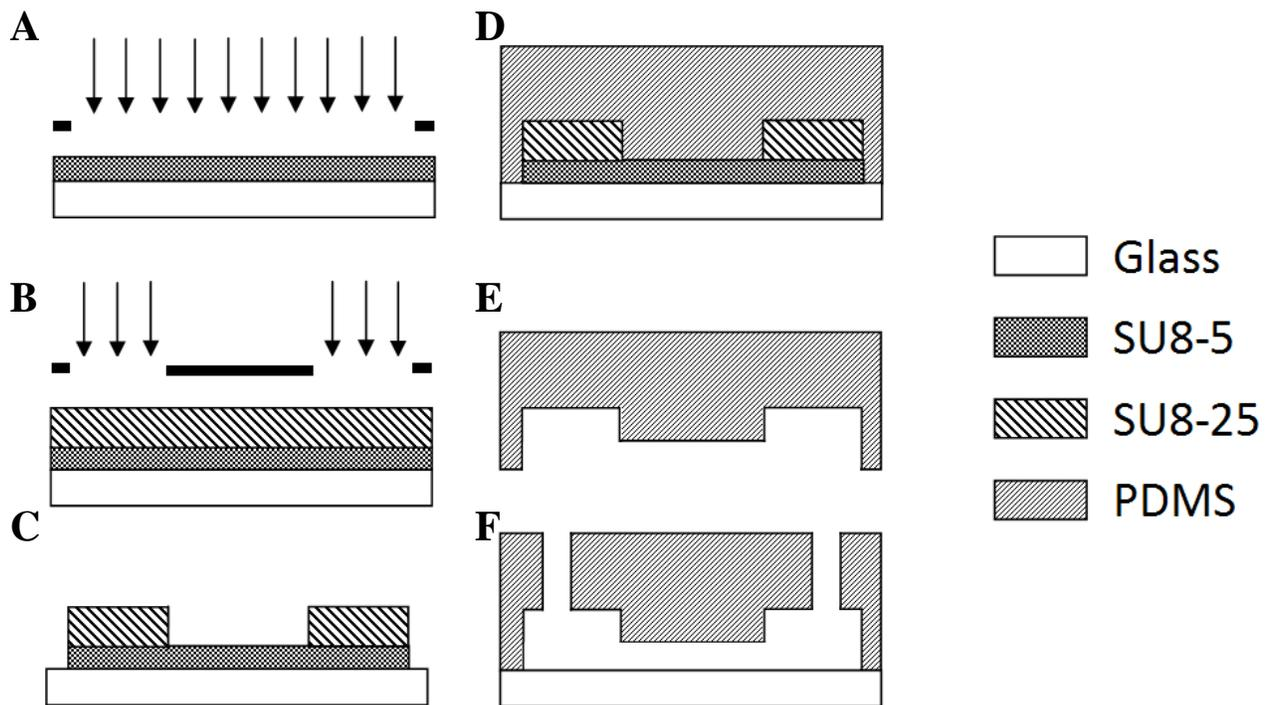
Supplementary Figure S.1: Fabrication of the two-layer PDMS device. Two layers of SU-8 were used to form mold masters.
