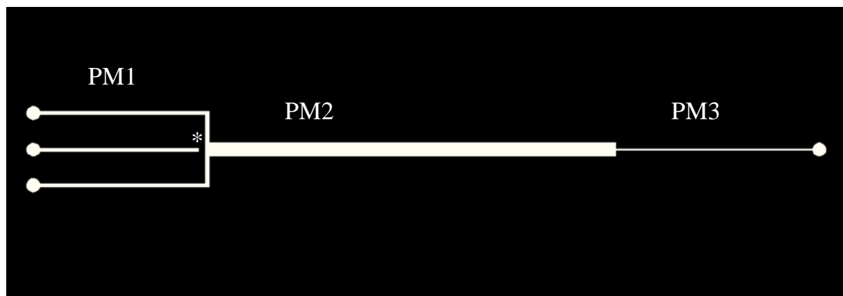
Fig. S2. Photomasked for device in ESI Fig.S3. The device is of basic hydrodynamic focusing design save for Disconnected Photomask Feature (*) for the center channel that eventually becomes an orifice after BDLL. Photomask dimensions. PM1 L: 10.5 mm, PM1 W: 300 \mu m, PM2 L: 27 mm, PM2W: 1 mm, PM3 L: 13 mm, PM3 W:150 \mu m.
