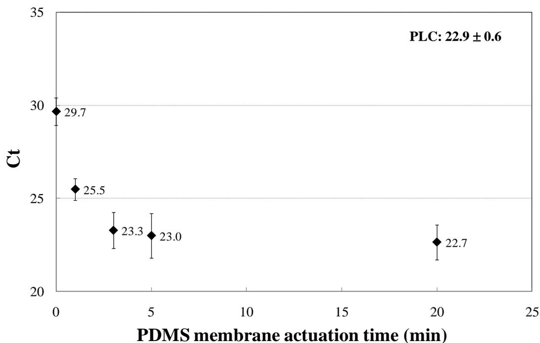
**Supplementary Figure S4.** Ct values as a function of PDMS membrane actuation time. 1 mL of *S. aureus* ( $10^6$  CFU/mL) was applied. Three repetitions were performed for each actuation time.
