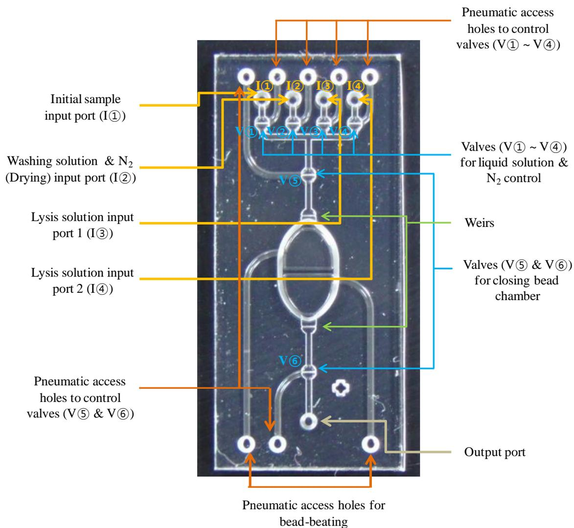
**Supplementary Figure S2.** Detailed description of microfluidic components in bead-beating microdevice.
