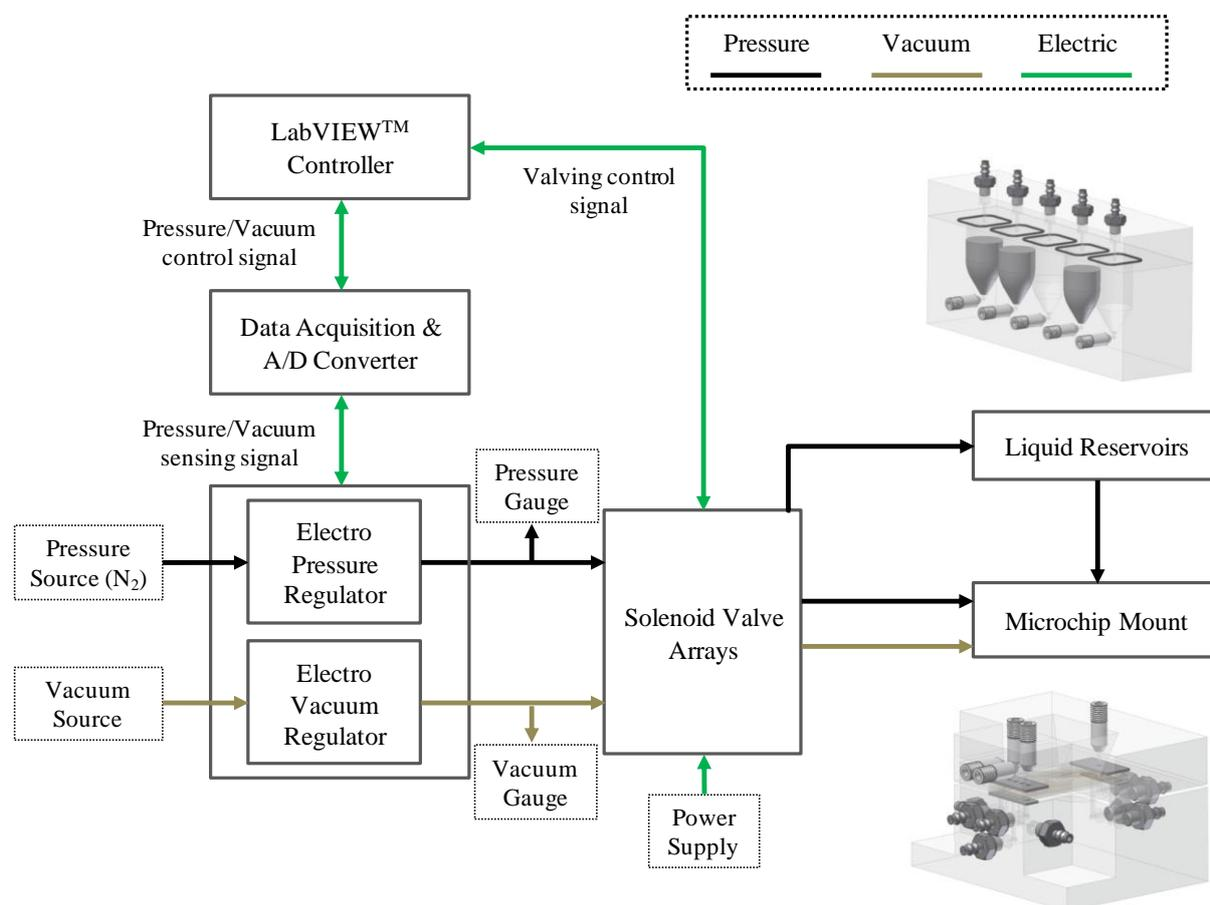
Supplementary Figure S1. Experimental set-up for the automatic extraction of bacterial DNA.
