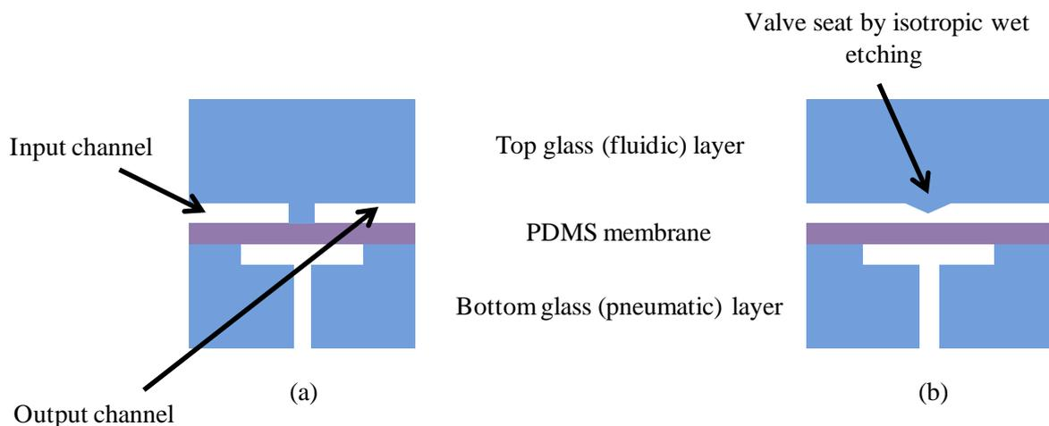
**Supplementary Figure S3.** Cross-sectional illustration view of the membrane valve structure: (a) PDMS sticking onto valve seat (normally-closed type) with plasma-activated permanent bonding, and (b) isotropically-etched valve seat (normally-half-open type) to prevent PDMS sticking
