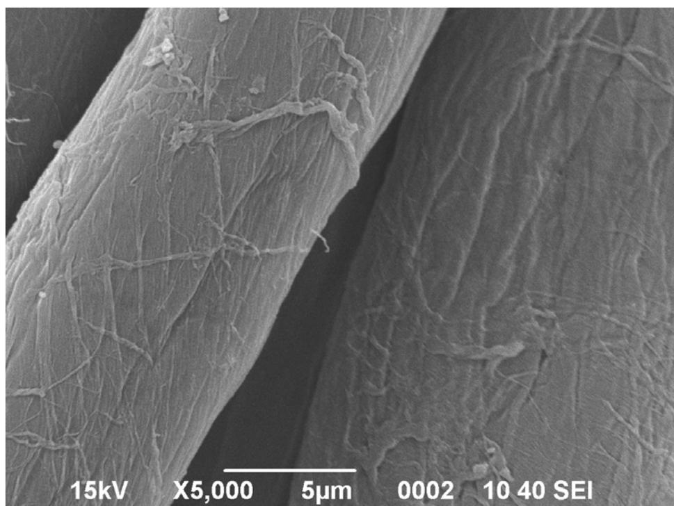
**Figure S2.** Secondary electron image (SEI) SEM image of cotton fiber after NaOH scouring/mercerization, showing the underlying spiral winding cellulose with some remain of the non-cellulosic materials
