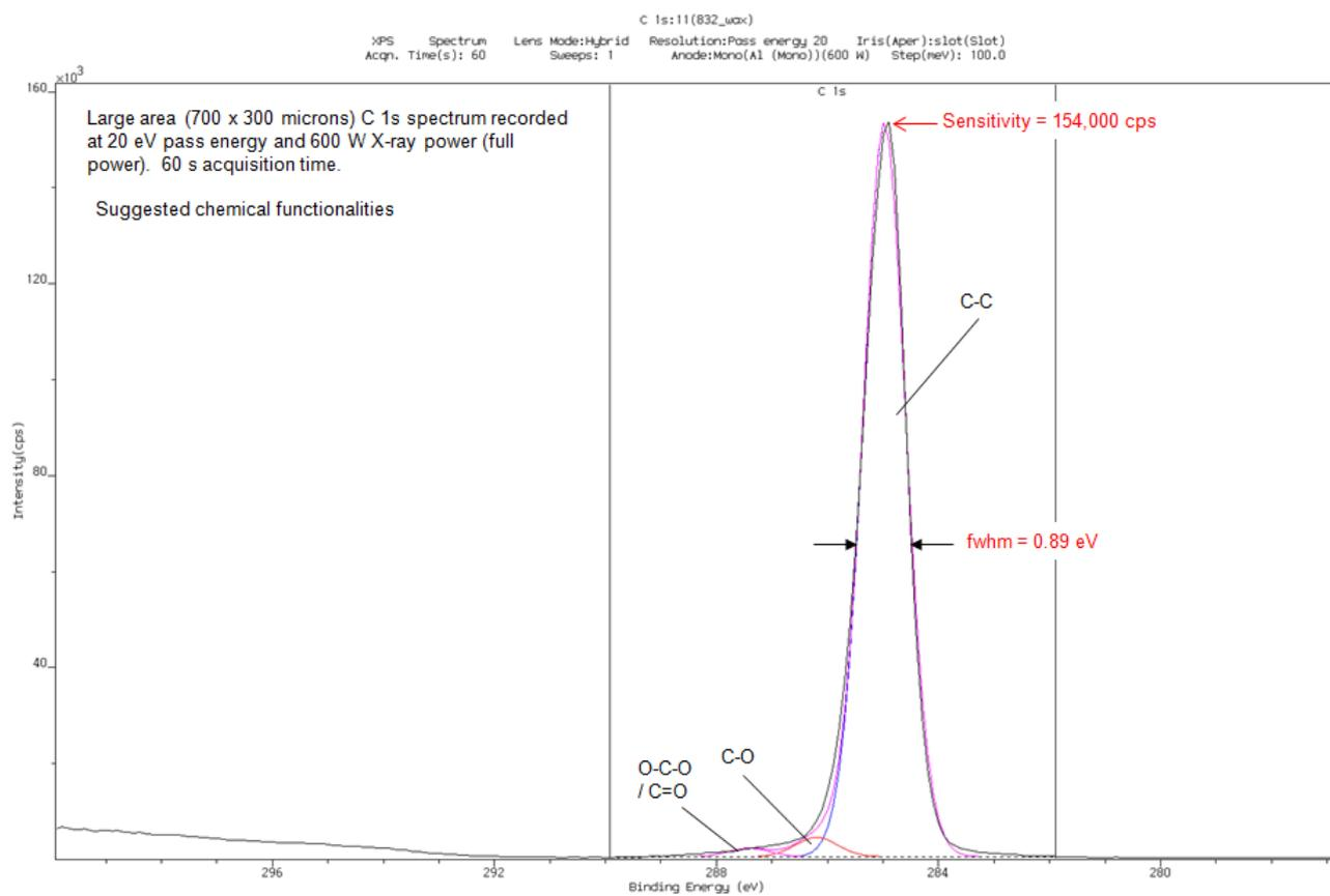
**Figure S10.** C 1s peaks from the XPS spectra of Waxed Cotton Cloth.
