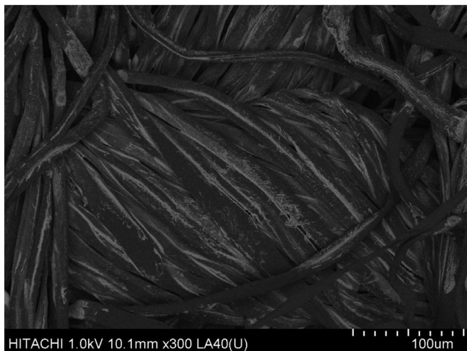
**Figure S6.** Low-angle backscattered electron image (LA-BE) FESEM image of silver (Ag) nanoparticle ink flow into Na<sub>2</sub>CO<sub>3</sub>-scoured cotton fabrics. Brighter parts indicate the Silver element which has heavier atomic weight.
