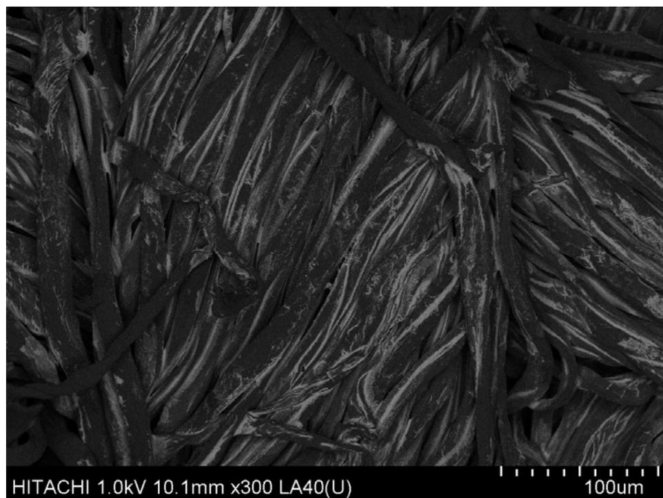
**Figure S5.** Low-angle backscattered electron image (LA-BE) FESEM image of silver (Ag) nanoparticle ink flow into NaOH-scoured cotton fabrics. Brighter parts indicate the Silver element which has heavier atomic weight.
