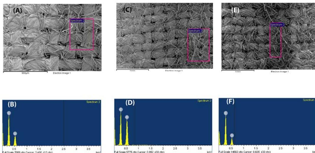
**Figure S7.** SEM and the corresponding EDS spectra of the unwaxed regions in untreated (A)-(B), NaOH-scoured (C)-(D), and Na<sub>2</sub>CO<sub>3</sub>-scoured (E)-(F) cotton fabrics, respectively.
