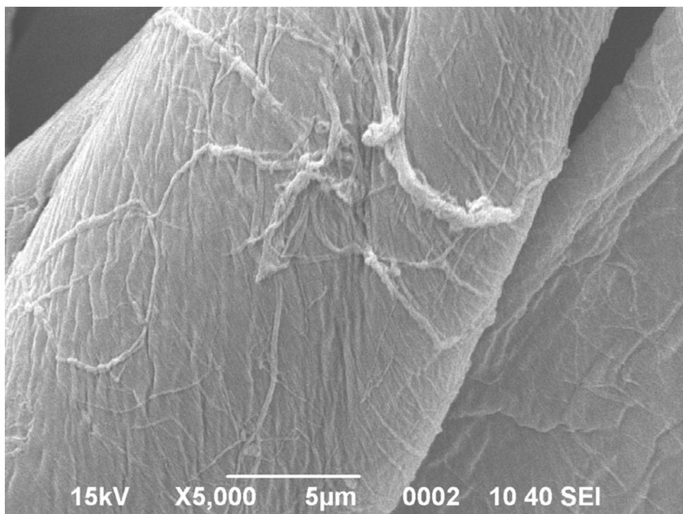
**Figure S3.** Secondary electron image (SEI) SEM image of cotton fiber after Na<sub>2</sub>CO<sub>3</sub> scouring/bleaching, showing the underlying spiral winding cellulose with some remain of the non-cellulosic materials, similar as the result of NaOH scouring
