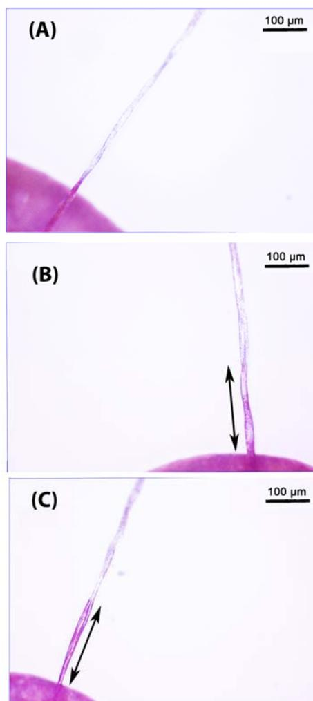
**Figure S11** Wicking of red ink in single fiber of untreated (A), NaOH-scoured (B), and Na<sub>2</sub>CO<sub>3</sub>-scoured (C) cotton. The red curve at the bottom of each picture is the 100 nl ink droplet reservoir
