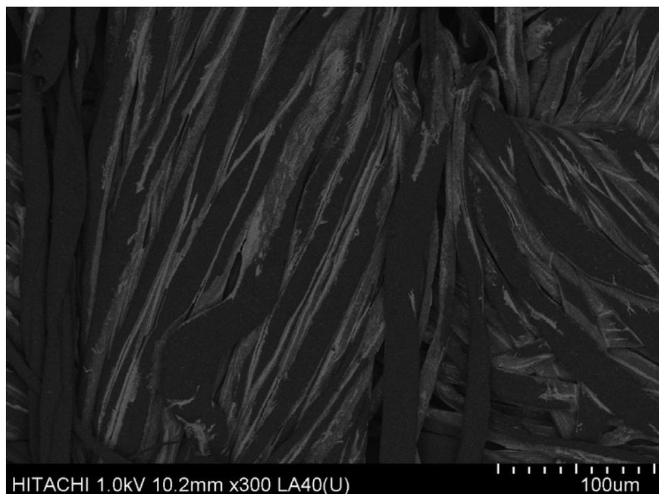
**Figure S4.** Low-angle backscattered electron image (LA-BE) FESEM image of silver (Ag) nanoparticle ink flow into untreated cotton fabrics. Brighter parts indicate the Silver element which has heavier atomic weight.
