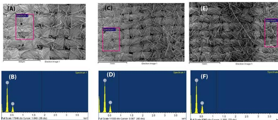
**Figure S8.** SEM and the corresponding EDS spectra of the waxed regions in untreated (A)-(B), NaOH-scoured (C)-(D), and Na<sub>2</sub>CO<sub>3</sub>-scoured (E)-(F) cotton fabrics, respectively.
