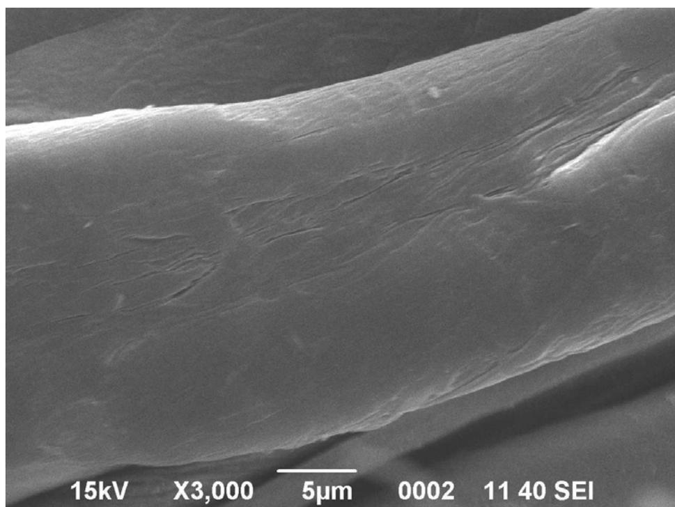
**Figure S1.** Secondary electron image (SEI) SEM image of cotton fiber before scouring, showing an outer layer of natural wax on its wall
