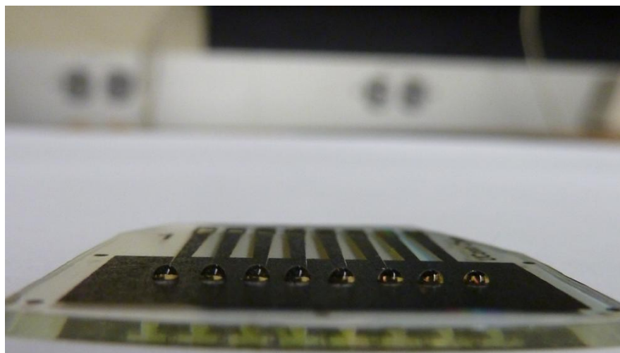
Supplementary Figure S2. Side view of the finished sensor array with 1 \mu\text{L} droplets of PBS contained by the hydrophobic microwell on each sensor spot.
