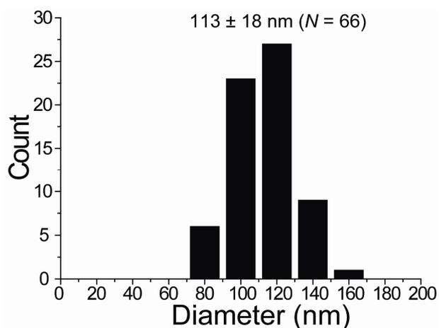
**Fig. S1** The histogram of the core diameter of nanothermometers determined by the transmission electron microscopy. Numbers at the top indicates the average  $\pm$  S.D. ( $N$ , the number of particles analyzed).
