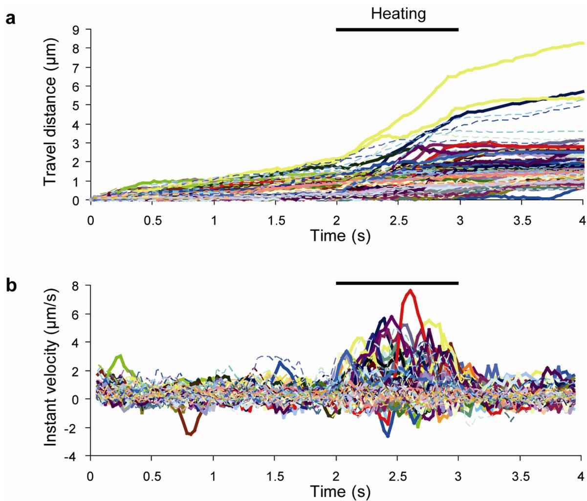
**Fig. S6** (a) Travel distance of each nanothermometer. (b) Instant velocities of nanothermometers in (a). Instant velocities were calculated as the travel distance per 150 ms.
