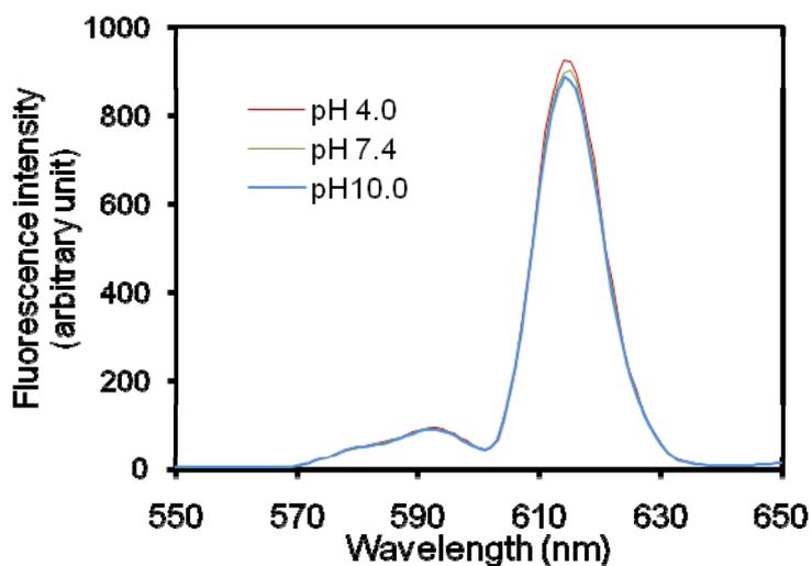
**Fig. S3** Fluorescence spectra of nanothermometer in PBS buffer (pH = 4.0, 7.4 and 10.0) at Ex. 341 nm.
