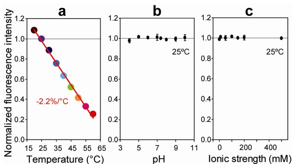
**Fig. S2** Properties of nanothermometer. (a) Relationship between the fluorescence intensity and the temperature. The red line indicates the linear fit with a slope of -2.2%/°C. (b) Fluorescence intensity at various pH. (c) Fluorescence intensity at various ionic strengths. In (a–c), the fluorescence intensities are represented as relative values against 25°C, pH 7.4 and 150 mM, respectively. Fluorescence intensity was measured at Ex. 341 nm and Em. 613 nm.
