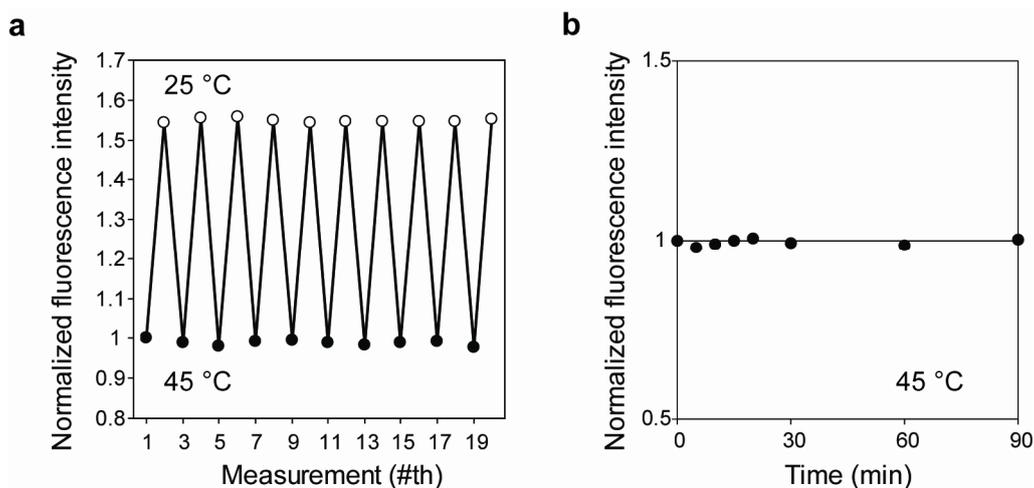
**Fig. S4** (a) Fluorescence intensity of nanothermometers which is reversible and repeatable against the temperature changes between 25°C and 45°C. (b) Stability of fluorescence intensity at 45°C. Fluorescence intensity was measured at Ex. 341 nm and Em. 613 nm.
