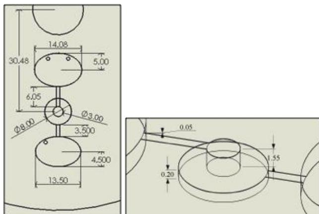
Figure S1. Dimensions of design used for initial dissolvable film plug validation.
