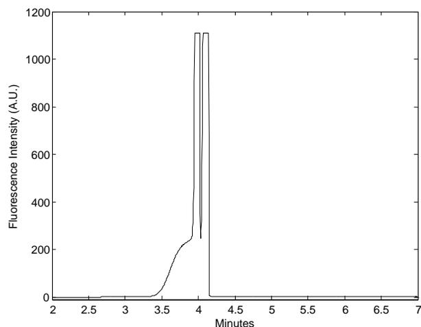
**Fig. 7** Capillary-ITP result for a 0.12  $\mu\text{L}$  sample containing glutamate-FITC and phenyl alanine-FITC both 50  $\mu\text{mol/L}$ . The measurement using LIF shows from left to right, Phe-FITC and Glu-FITC, shown to be concentrated so far as to saturate the detector ( $>250 \mu\text{mol/L}$ ).
