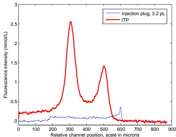
**Fig. 9** ITP result in a 330 nm deep channel. Based on the areas under the curves, the ITP result corresponds to an injection of 3.2 pL. This larger injection volume resulted in higher peaks and more spacing compared to the 0.4 pL sample in Figure 2c.
