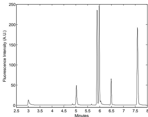
**Fig. 5** Typical CZE electropherogram of labeled amino acids and FITC by-products. From left to right first at 3 minutes the EOF marker bodipy is seen, then FITC-ethanol, leucine-FITC, phenyl alanine-FITC, fluorescein amine-FITC and glutamate-FITC, all except FITC-Ethanol at 10  $\mu$ mol/L.
