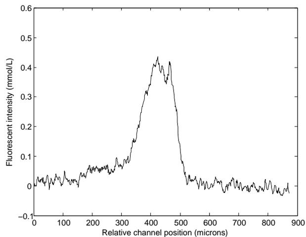
**Fig. 10** ITP focussing result in a 330 nm deep channel, part of the same experiment as in Figure 2. The applied voltage difference of 200V ( $A = 100$  V,  $F = -100$  V).
