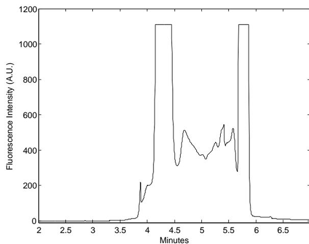
**Fig. 6** Capillary-ITP for a 0.12 µL sample of yeast biomatrix and 5 glutamate-FITC and phenyl alanine-FITC both 50 µmol/L. The measurement using LIF shows from left to right, Phe-FITC and Glu-FITC, spaced by the yeast biomatrix, with TE to the left and LE to the right of the sample.
