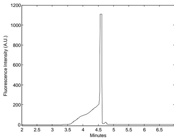
**Fig. 12** Graph showing the capillary-ITP result with 50  $\mu\text{mol/L}$  phenyl alanine-FITC same protocol as used for Figure 6.
