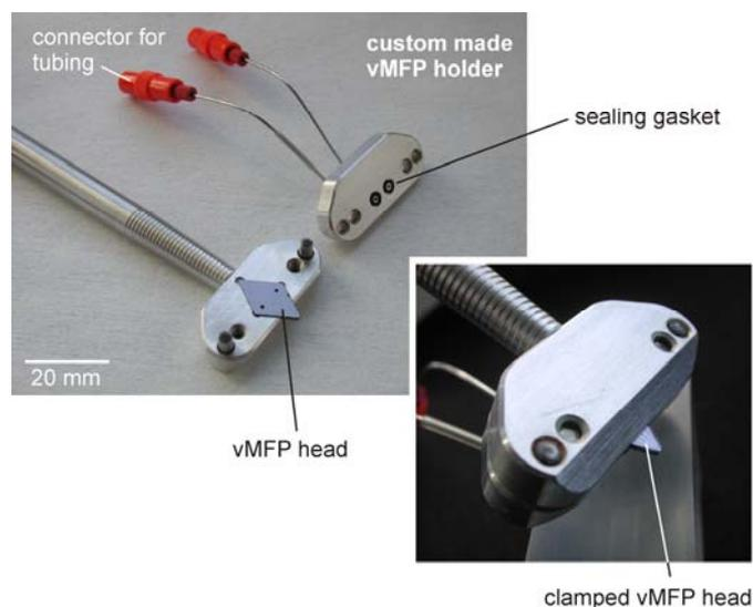
The vMFP head was mounted within a custom aluminum holder prior to performing an experiment. The head holder is shown here with a vMFP head before and after assembly. The syringe pumps (not shown) were connected to the holder through capillary tubing. O-rings were used to seal the connection between the vias of the vMFP head and the ports in the holder. If required, replacement and leveling of the vMFP head over a sample/tissue section was done within minutes.
