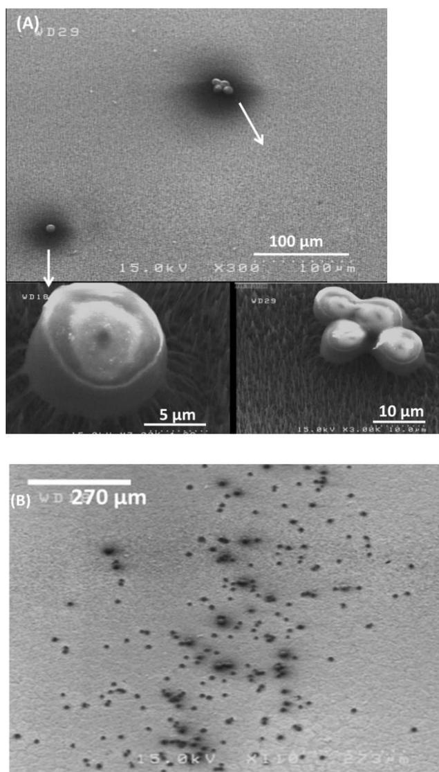
Figure 1S. SEM image from the entrapment of (A) fixed and (B) live SW48 cancer cells with the same concentration on MWCNT arrays. The fraction of entrapped fixed cells is observably lower than live ones.
