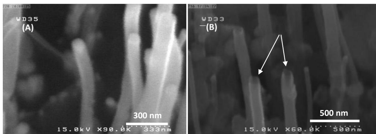
Figure 2S. High magnification SEM images of, (A) Ni/MWCNT in which the Ni has a dome shape.
