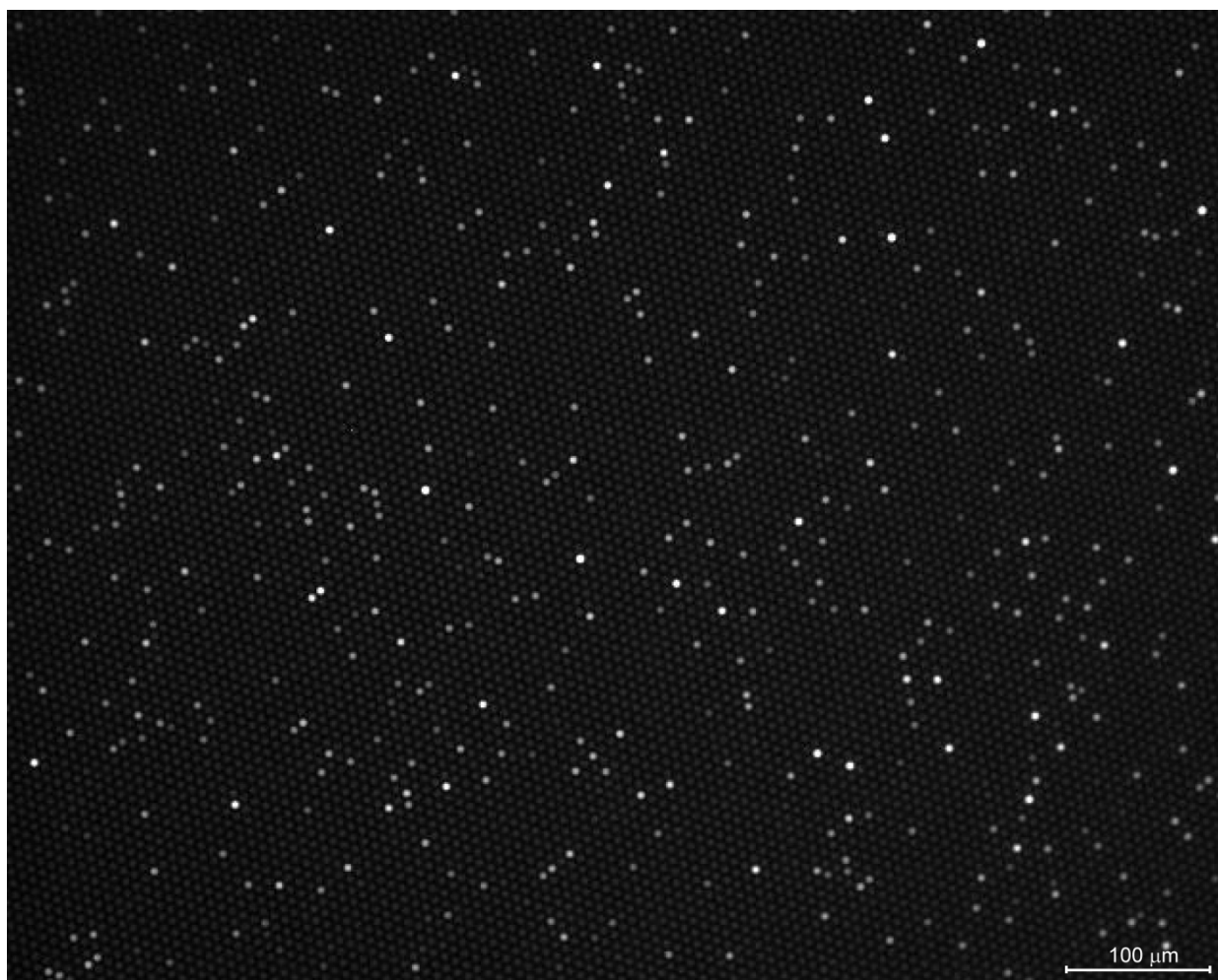
Fig. S1. On-chip sealing using mineral oil. A section of the femtoliter microwell array after an enzyme/substrate solution containing 0.72 pM \beta -gal and 100 \mu M RDG has been sealed by mineral oil with an on-chip protocol. The accumulation of fluorescent product in wells containing an active enzyme molecule makes them clearly distinguishable from the background.
