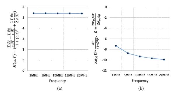
**Figure S4** Factors proportional to velocities of electrothermal- and electroosmotic flows in terms of frequency variation (a) M factor for electrothermal flow (b)  $\frac{a^2}{(1+a^2)^2}$  for electroosmotic flow. This parameter is the dominant variable of time-averaged AC electroosmotic velocity.
