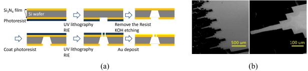
Figure S1. (a) Microtip fabrication procedure. (b) SEM images of the microtips.
