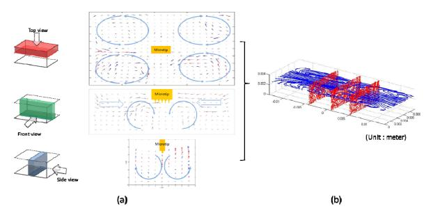
**Figure S3.** (a) PIV analysis of 2 dimensional flow for each plane, which is generated by longitudinal vibration of an aluminum well. (b) 3 dimensional flow that is generated by combining 2 dimensional flows.
