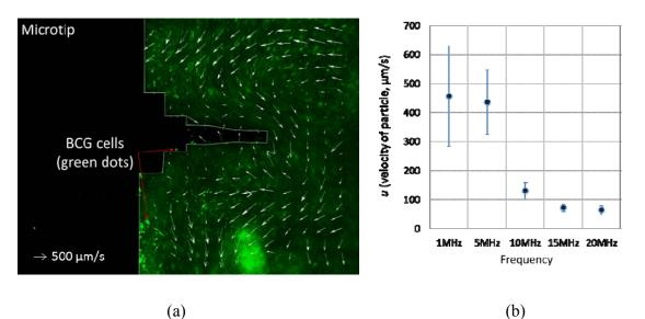
**Figure S5.** Motion of BCG cells under an AC e-field (5MHz at 20  $V_{pp}$ ). (a) Stained BCG cells were circulated around the microtip due to EHD flow and attracted on the surface of a microtip by DEP. (b) Average velocities of EHD flow in the vicinity of a microtip according to frequencies.
