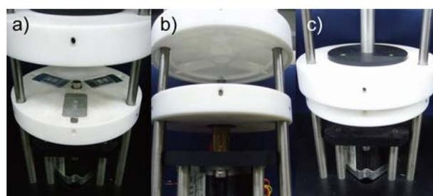
**Fig. S2** Digital image for a Rotary Genetic Analyzer platform: a) Top view showing the Rotary stage which incorporates three thermal blocks, b) bottom view showing an upper teflon cover with block-shaped hollow, and c) a tightly sealed Rotary PCR system for thermal cycling.
