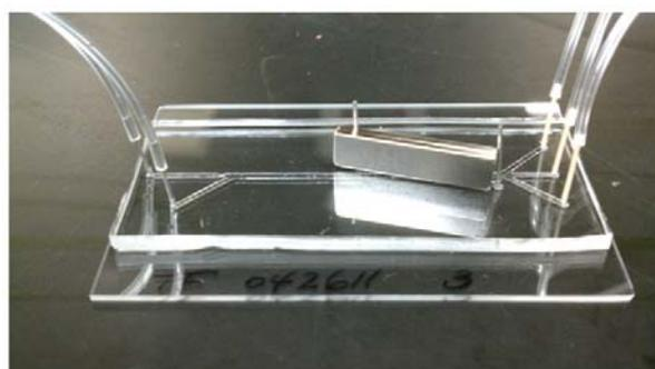
FIG. S7. PDMS microfluidic device for magnetophoretic displacement measurements.
