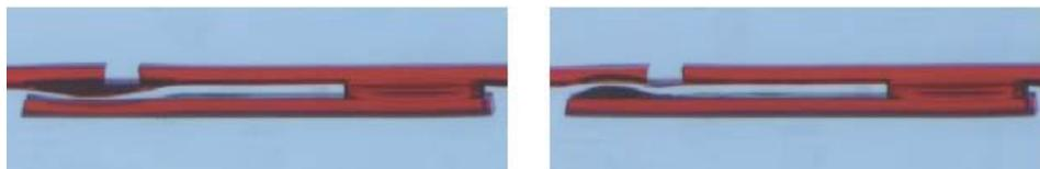
(2) Nanoliter range aqueous plugs (red) are transferred by squeezing an oil-filled reservoir (left) connected with two check valves through a T-junction (also see Fig. 4b).
