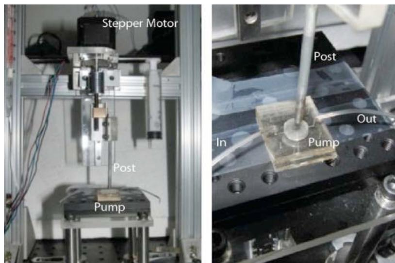
**Fig. S5** The homebuilt apparatus for performance test of a pump. A computer was used to control the stepper motor, which drove the dome-headed post to push the chip. The diameter of the metallic post is 2mm, and the squeezing/releasing speed is 1.2 mm/s.
