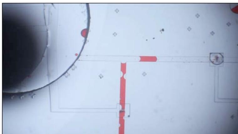
(3) Operation of a squeeze chip. Dyes are used to demonstrate the liquid flow driven by the pump actuations.
