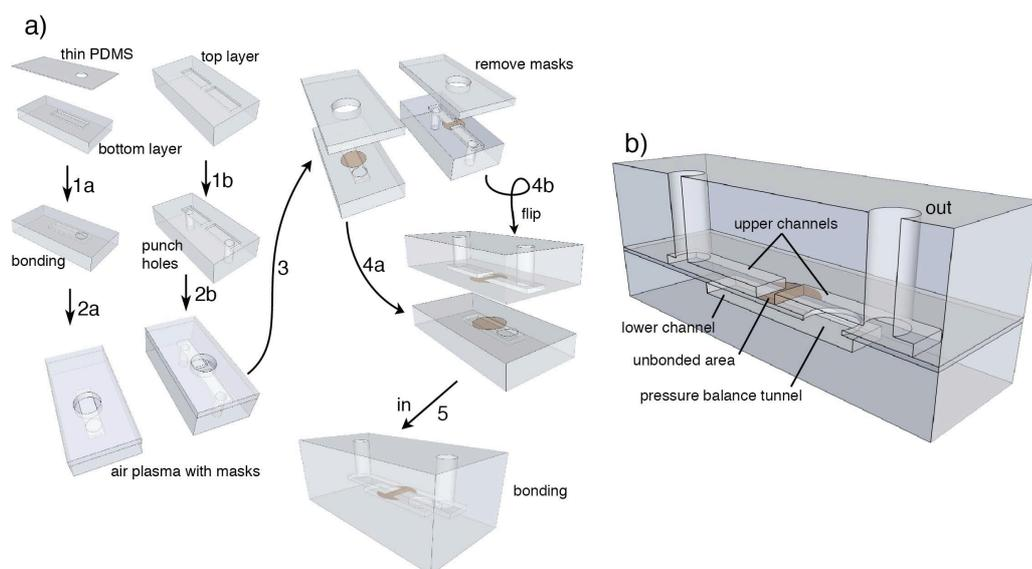
**Fig. S1** The monolithic PDMS check valves. a) Fabrication of a check valve. b) Structure of a check valve. A deformable membrane section, created by oxidization of the PDMS surface through air plasma treatment, is the key component of the valve.
