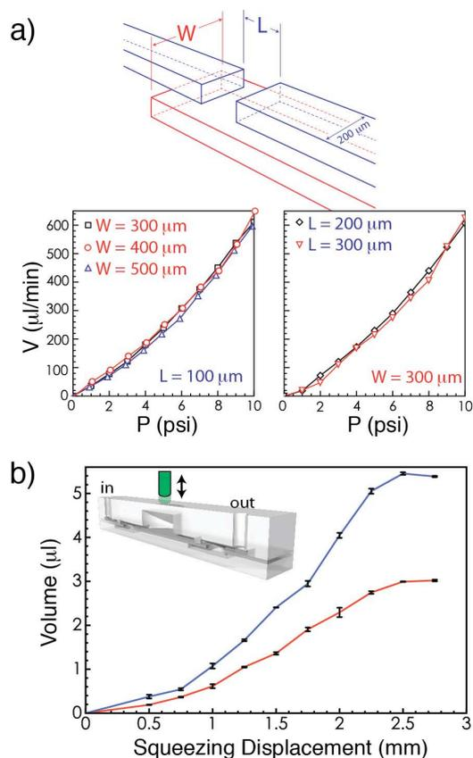
**Fig. S4** a) The flow velocity of water through the valves is not sensitive to structure variation. b) Volume per squeeze measured from a chip (reservoir is 1 cm in diameter and 3 mm thick). 1s dwell time between the squeezes (blue line) offers better pump efficiency than continuous squeezes (red line).
