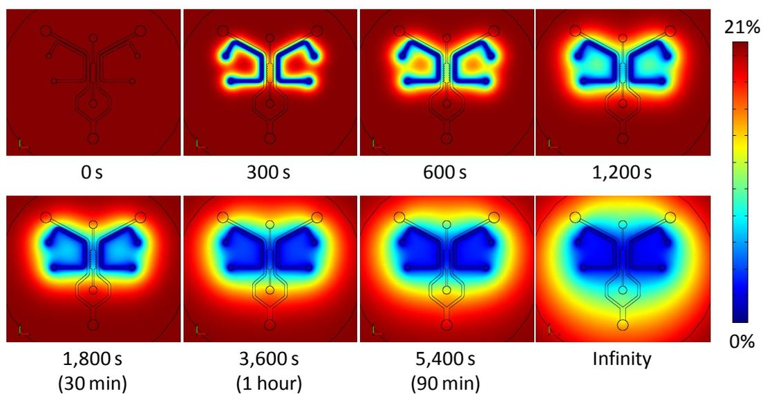
**Figure S4.** Transient change of oxygen tension on a crosssection ( $z = 1.0 \times 10^{-6}$  m) of the microfluidic device with a film of low diffusion coefficient ( $D_{\text{film}} = 2.0 \times 10^{-12}$  m<sup>2</sup>/s), supplying 0% oxygen gas to both gas channels.
