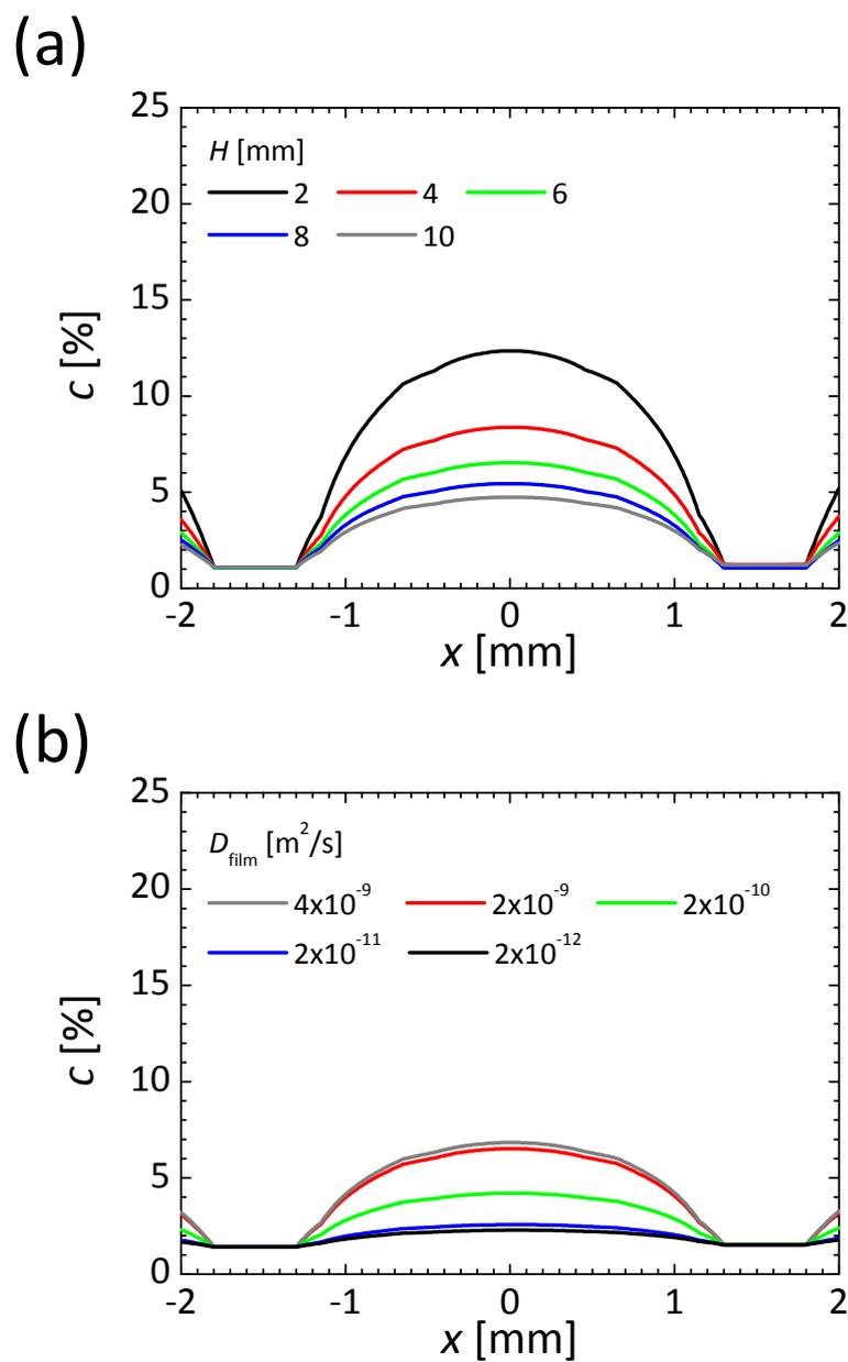
**Figure S3.** Variations of oxygen tension profile across the middle of the gel region,  $(y, z) = (1.975 \times 10^{-3} \text{ m}, 1 \times 10^{-6} \text{ m})$ , in the microfluidic device at media and gas flow rates of  $(Pe_m, Pe_g) = (10, 100)$  with parameters: (a) the device of different thickness without a film, and (b) the device with a film of different diffusion coefficient of oxygen ( $H = 6$  mm).
