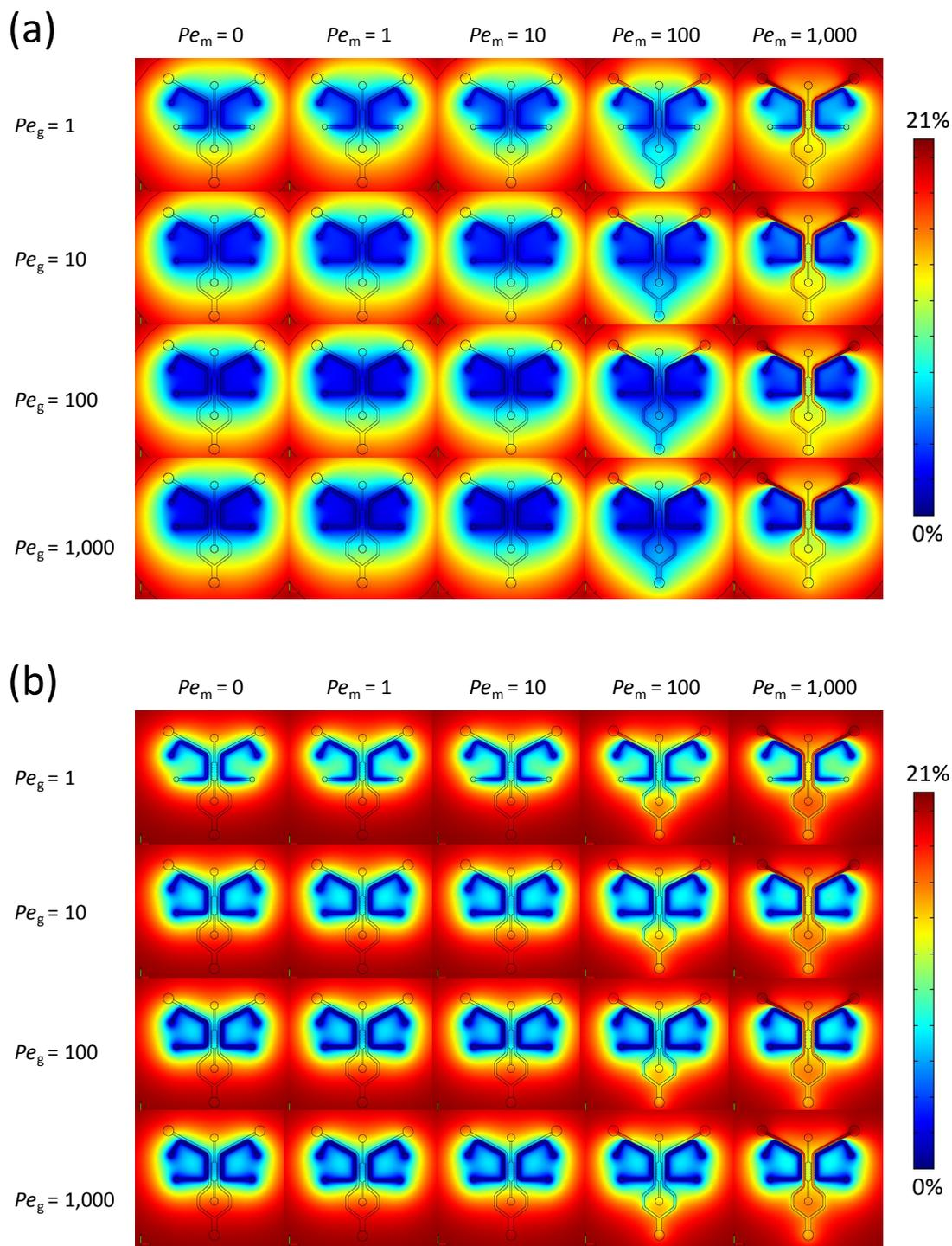
**Figure S2.** Variations of steady oxygen tension on a crosssection ( $z = 1.0 \times 10^{-6}$  m) of the microfluidic devices (a) with and (b) without a film of low diffusion coefficient of oxygen ( $D_{\text{film}} = 2.0 \times 10^{-12}$  m<sup>2</sup>/s) with a combination of Péclet numbers for media and gas flow, supplying 0% oxygen gas to both gas channels.
