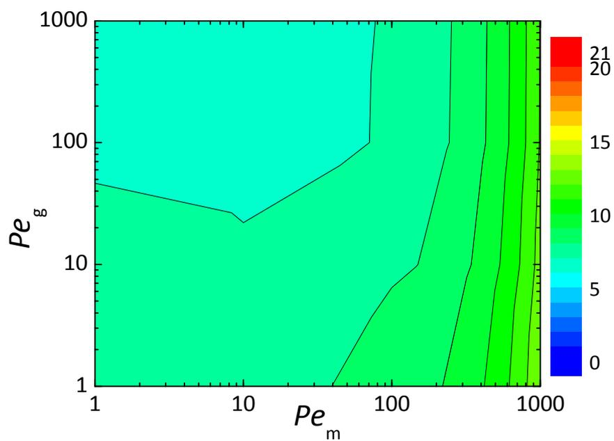
**Figure S1.** Contour map of oxygen tension at the center of the gel region on a glass cover slip,  $(x, y, z) = (0 \text{ m}, 1.975 \times 10^{-3} \text{ m}, 1 \times 10^{-6} \text{ m})$ , in the microfluidic device without a film with a combination of Péclet numbers for media and gas flow, supplying 0% oxygen gas to both gas channels.
