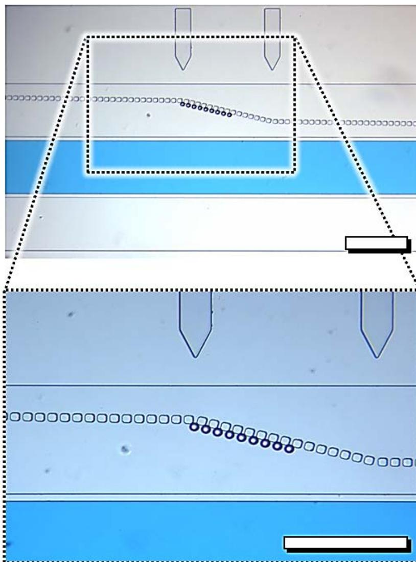
**ESI Figure 6** Experimental results for varying  $\alpha$  from  $1^\circ$  to  $15^\circ$  to  $1^\circ$  in order to immobilize a select number of microbeads within a  $\mu$ PAR system. Scale Bars =  $200\ \mu\text{m}$ .
