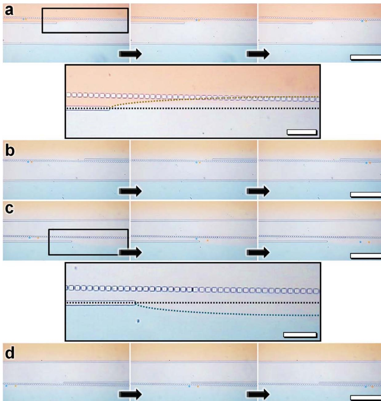
**ESI Figure 4** Experimental results for limiting biotin and avidin diffusion into the wash solution within the multiplexed  $\mu$ PAR system. **(a, b)** Suspended streptavidin-coated polystyrene microbeads ( $15\ \mu\text{m}$  in diameter) are transported from the biotinylated bovine serum albumin (BSA) solution (*yellow*) to the phosphate buffered saline (PBS) wash solution (*white*). The higher input flow rate for the PBS wash solution (*i.e.*, *versus*
