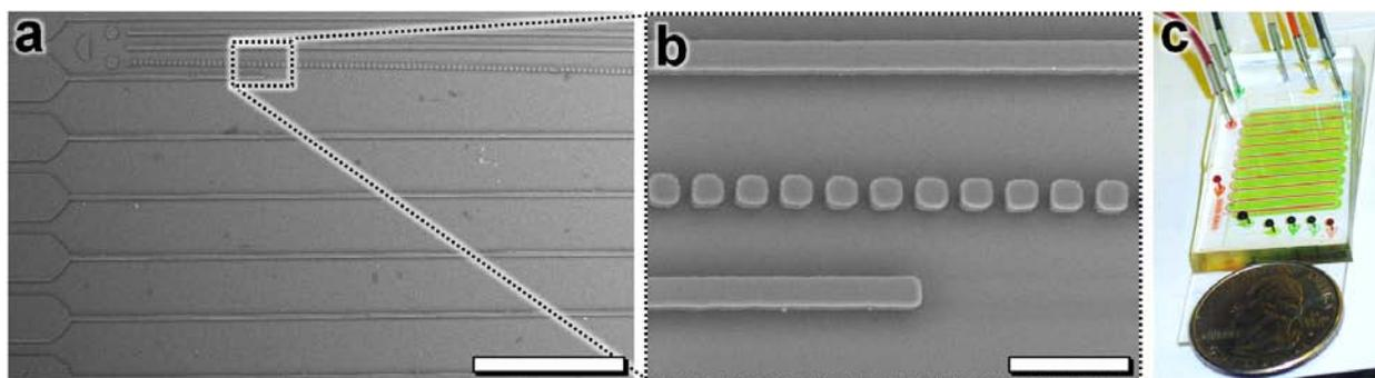
**ESI Figure 2** Microfabrication results for the multiplexed  $\mu$ PAR system. **(a, b)** SEM micrographs captured at magnifications of: **(a)** 100X, **(b)** 1,000X. **(c)** Photograph of the multiplexed  $\mu$ PAR system filled with coloured dye solutions next to a US Quarter (approximately 24.3 mm in diameter). Scale Bars = **(a)** 500  $\mu$ m, **(b)** 50  $\mu$ m.
