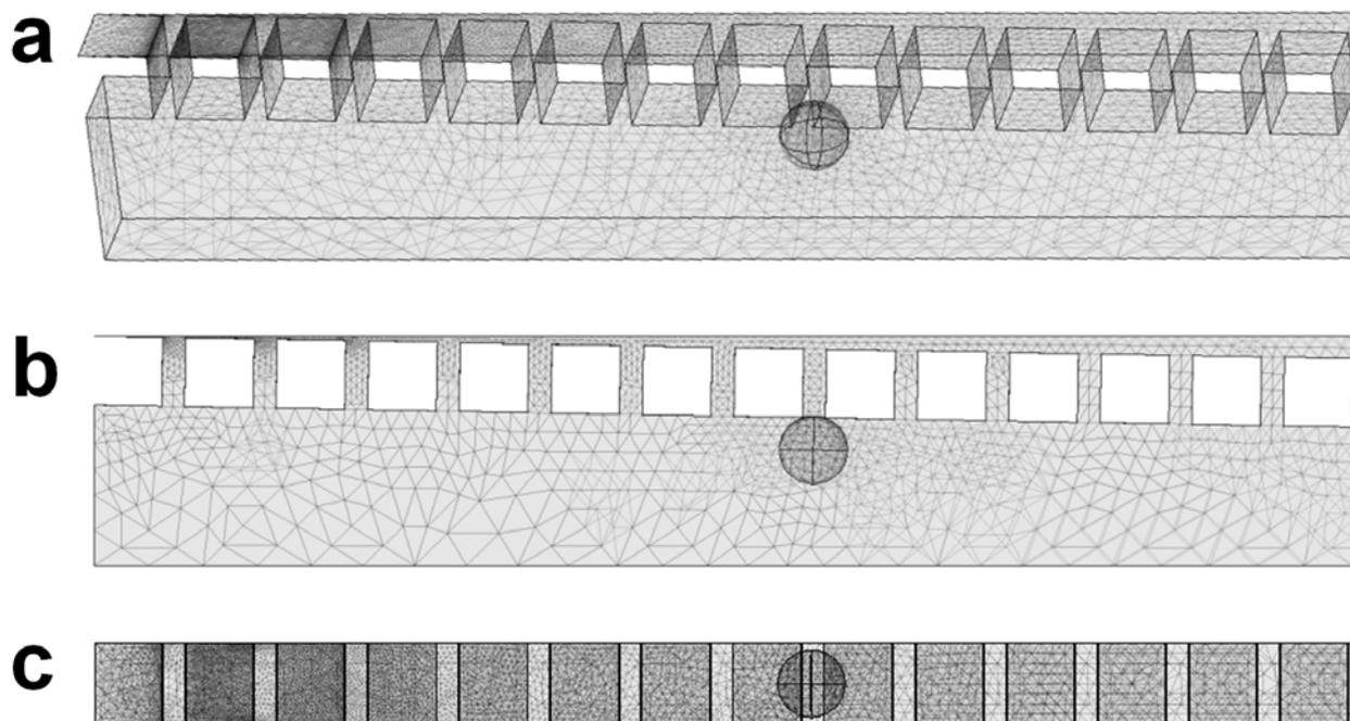
**ESI Figure 3** Expanded views of a meshed three-dimensional COMSOL Multiphysics model of a spherical microparticle ( $15 \mu\text{m}$  in diameter) immobilized within a  $\mu\text{PAR}$  system with  $\alpha = 1^\circ$ . **(a)** Three-dimensional view. **(b)** Top view. **(c)** Side view.
