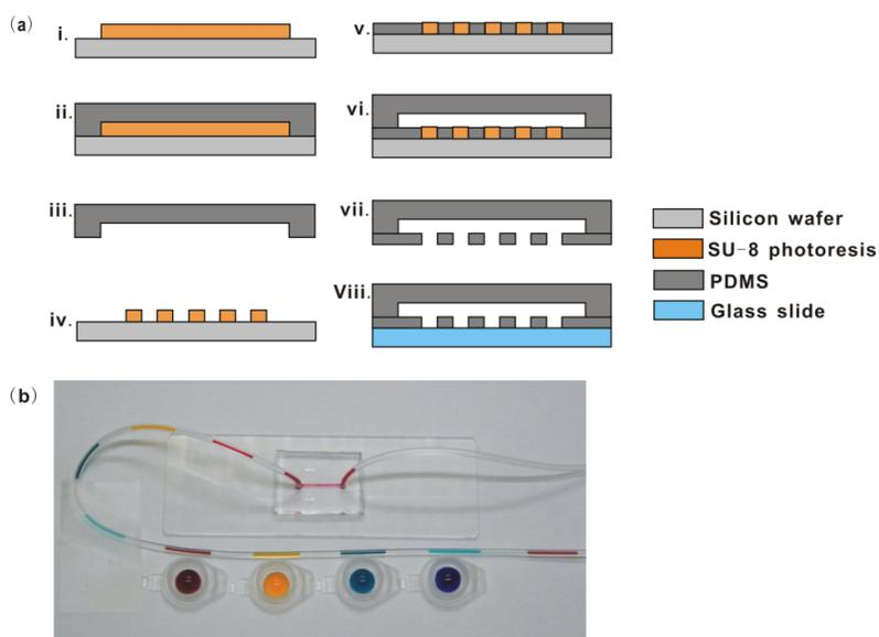
**Supplementary Fig. 2** (a) Flow diagram of fabrication procedure of the microfluidic device. (b) The photograph below showing the microdevice with pre-loading sequential gas-liquid plugs into a tubing for media isolation. The liquid plugs are filled with food dyes.
