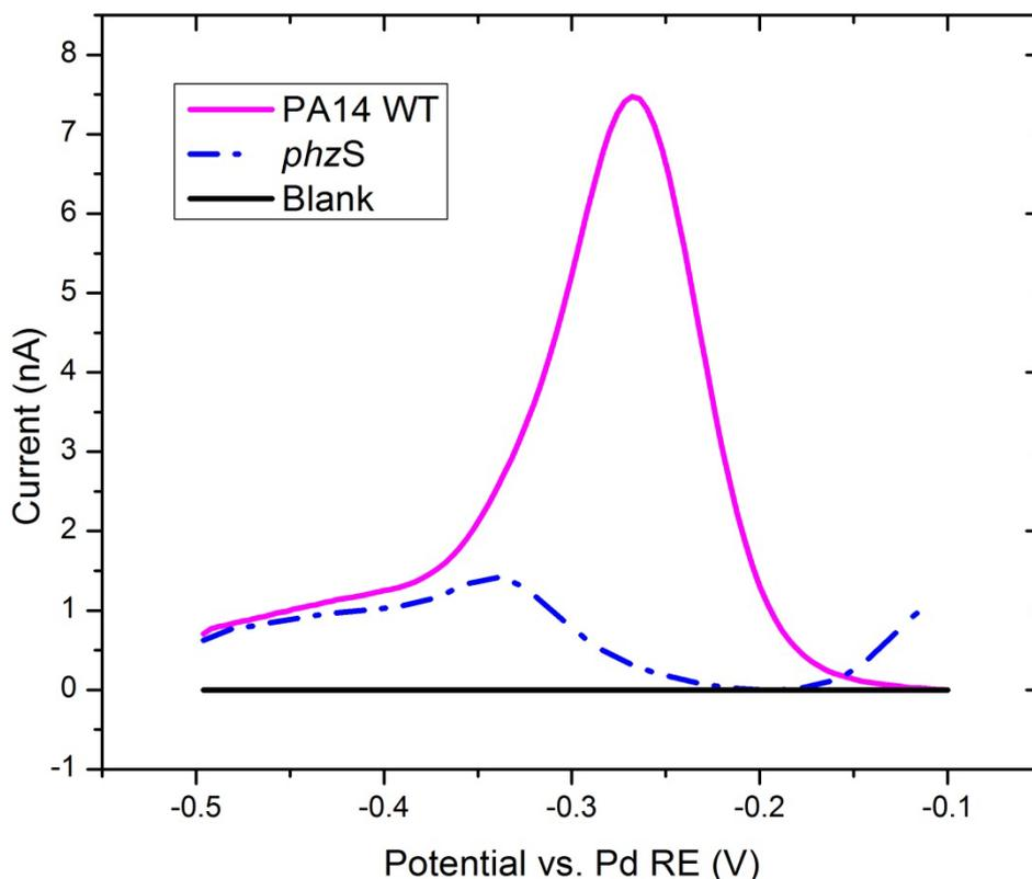
Figure S5: Differential pulse voltammogram of wild type PA14 and *phzS* after 6 days of growth at 37 °C. Scans were performed from -0.5 to -0.1 V at an amplitude voltage of 0.05 V and a frequency of 15 Hz.
