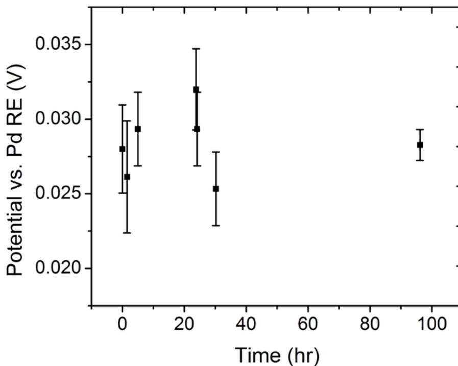
Figure S2: Oxidation potential of ferrocene dimethanol vs. a semi-charged PdH Re
