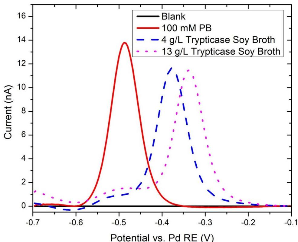
Figure S4: Differential pulse voltammograms of 100  $\mu\text{M}$  pyocyanin in Phosphate Buffer (Red Line) and in 4 g/L (Blue Dashed Line) and 13 g/L (Pink Dotted Line) Trypticase Soy Broth. Scanned at an amplitude voltage of 0.05 V and a frequency of 15 Hz.
