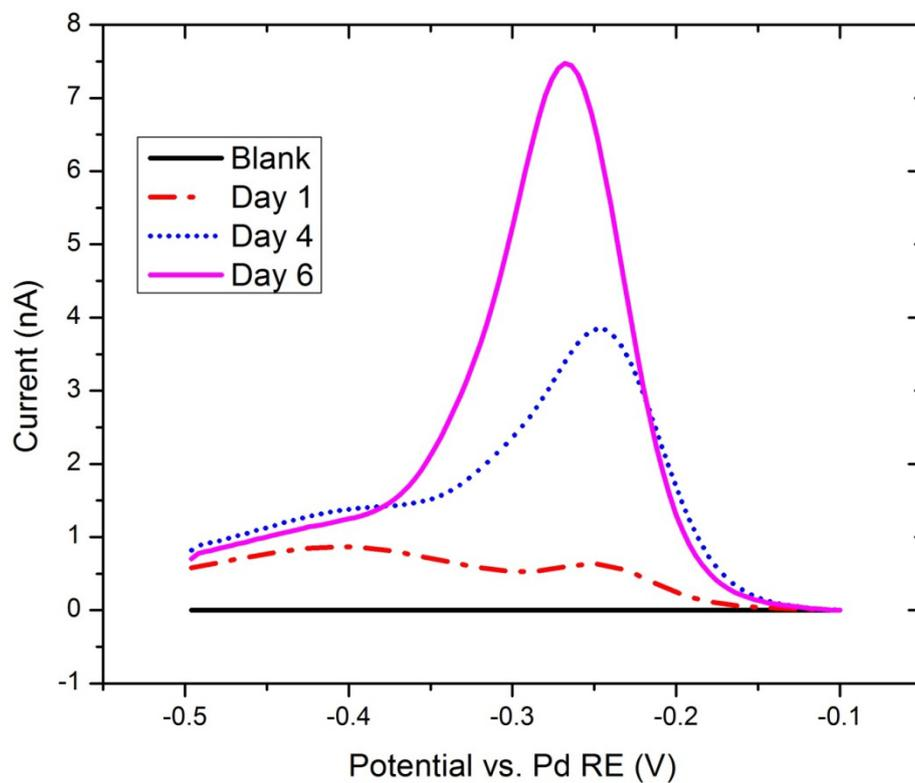
Figure S6: Differential pulse voltammograms of PA14 wild type supernatants over a 6 day period. Scans were performed from -0.5 to -0.1 V, at an amplitude voltage of 0.05 volts and a frequency of 15 Hz.
