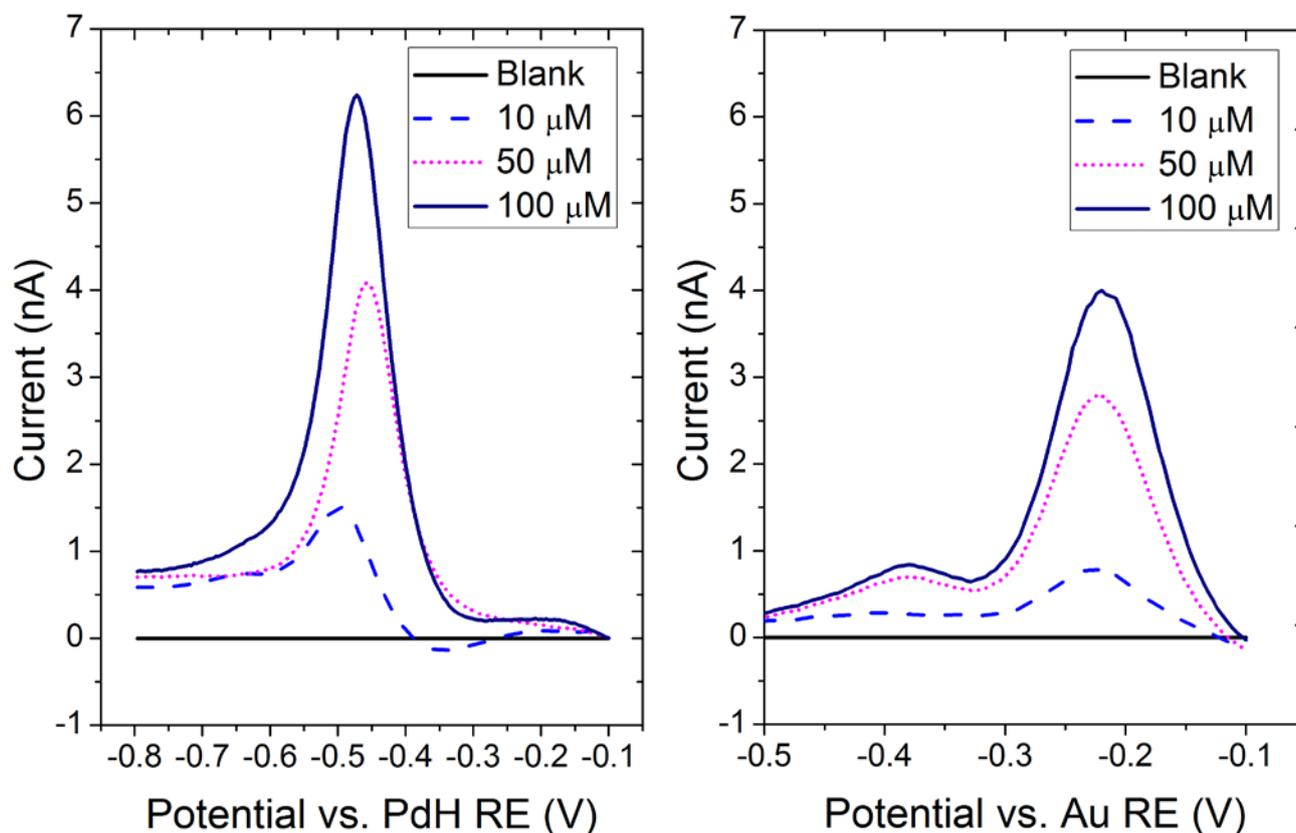
Figure S3: A) Differential pulse voltammograms of 0 - 100  $\mu\text{M}$  pyocyanin in 100 mM PB from -0.800 to -0.100 V vs. PdH reference electrode. B) Differential pulse voltammograms of 0 - 100  $\mu\text{M}$  pyocyanin in 100 mM PB from -0.500 to -0.100 V vs. Au reference electrode. All scans were performed at an amplitude voltage of 0.05 volts and a frequency of 15 Hz.
