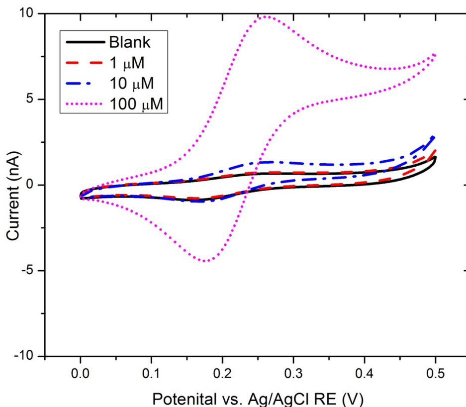
Figure S1: Cyclic voltammograms of 1-100  $\mu\text{M}$  ferrocene dimethanol in 1 M KCl solution. Scan rate of 0.050 V/s from 0 to 0.750 V using a Ag/AgCl reference electrode.
