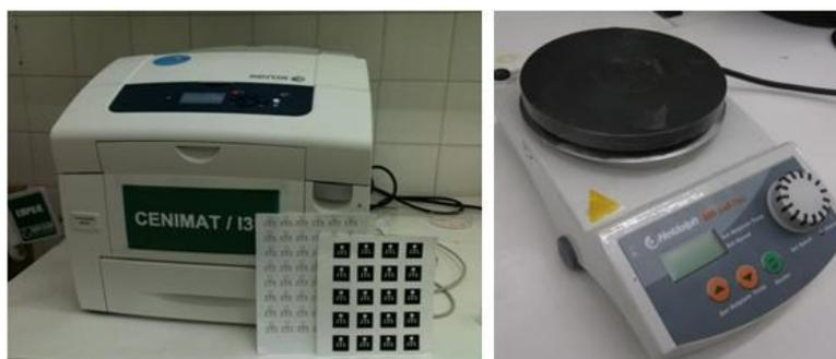
**Figure S4 – Equipment used for the fabrication of paper micro-plates: Xerox ColorQube solid ink Printer (left) and a thermal plate (right)**
