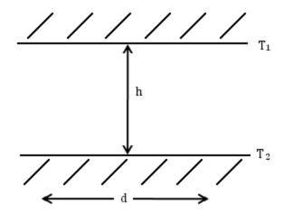
If  $T_2 > T_1$ , fluid is less dense near bottom  $\rightarrow$  creates a "top heavy" arrangement  $\rightarrow$  <u>unstable</u>
